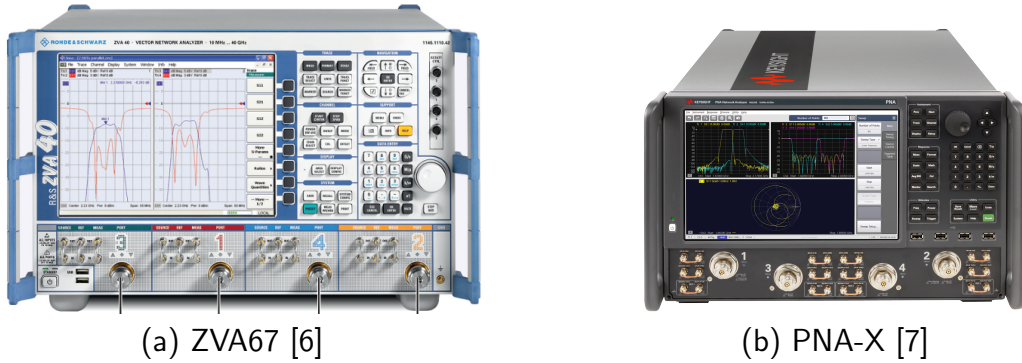
Figure 2.2: Commerical VNAs showing (a) ZVA67 by Rohde & Schwarz and (b) PNA-X by Keysight Technologies.
