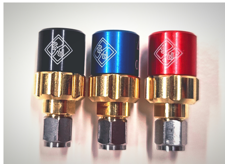
Figure 3.6: 1 mm coaxial calibration standards, match, open and short (from left to right) from Rohde & Schwarz ZV-Z210 calibration kit [5].
