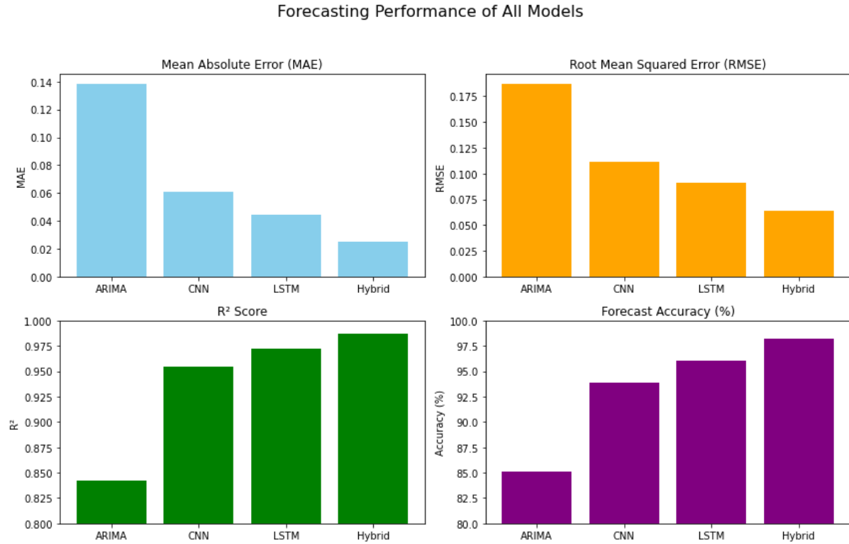
Figure 4.11: Forecasting performance comparison across ARIMA, CNN, LSTM, and Hybrid models based on MAE, RMSE, R^2 , and forecast accuracy. The Hybrid model demonstrates superior accuracy and consistency across all metrics
