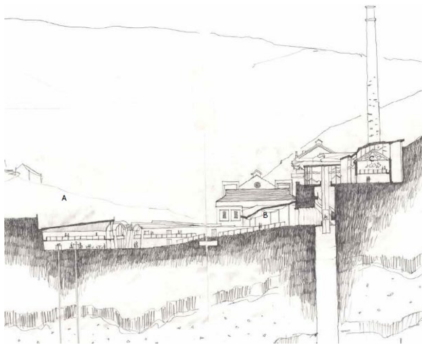
Figure 10. Cross section of proposal at Crumlin Navigation Colliery for Mine Water Heat Recovery Research Centre and National Coal Archives (McCormick, A., 2022)
