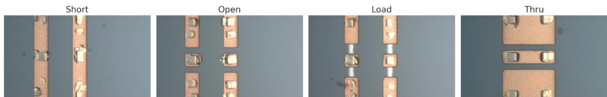
Figure 3.12 Optical microscope images of the SOLT (Short, Open, Load, Thru) calibration standards used for RF on-wafer calibration
