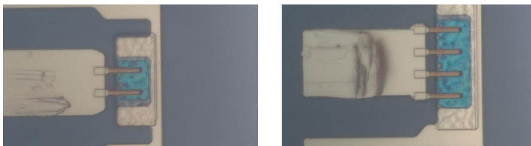
Figure 3.13 Optical micrograph of 2-finger/ 4-finger AlGaIn/GaN Schottky diode (GSG probing)
