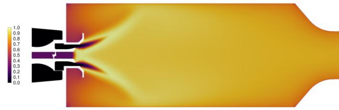
Fig. 3.4: Normalised temperature distribution predicted by CFD simulation
