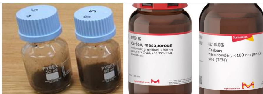
Figure 20: Photographs of the different carbonaceous powders tested (left: vials containing aircraft soot ‘scraped’ in different sections of a de-tuner, right: commercially available carbonaceous nanopowders)
