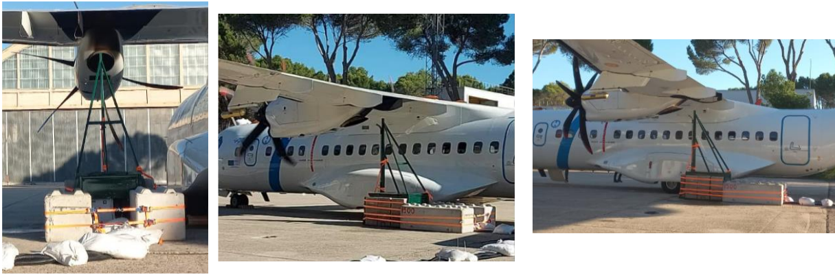
Figure 20: Pictures of the INTA dedicated probe and structure with concrete ballast used to weight down the structure
