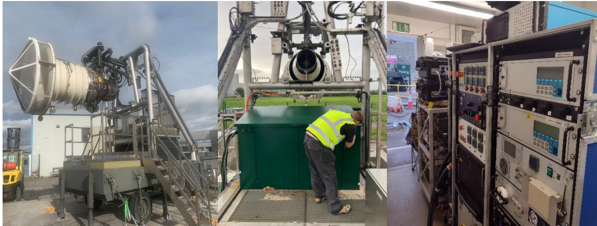
Figure 1: photographs of test engine on the CFS aero Hawarden test stand (left), sampling probe and near-field measurement cabinet (middle), and main measurement cabin (right)
