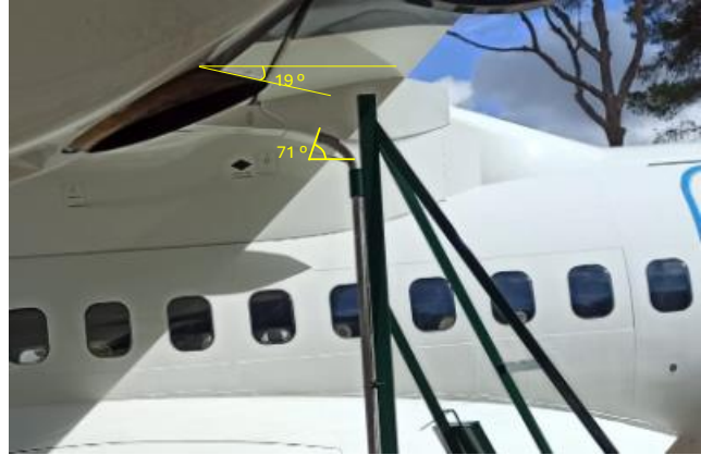
Figure 18: Diagram (left) and picture (right) of the dedicated INTAO probe orientation towards the engine exhaust
