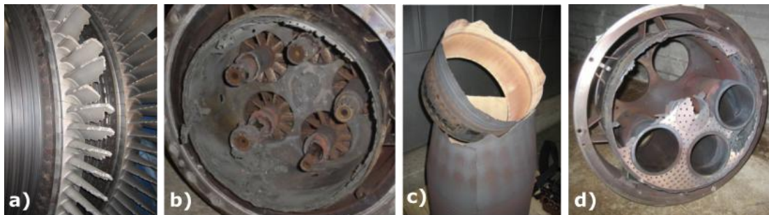
Figure 2.10 - Thermoacoustic instability induced damage in a turbine blade [a], burner assembly [b], gas turbine liner [c], combustor face plate [d]. (From Emmert [101] p.1 and Morgans [102] p. 8).
