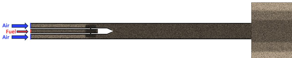
Figure 7.2 – Modified mesh for JICF burner with location of air and fuel mass flow inlets highlighted.
