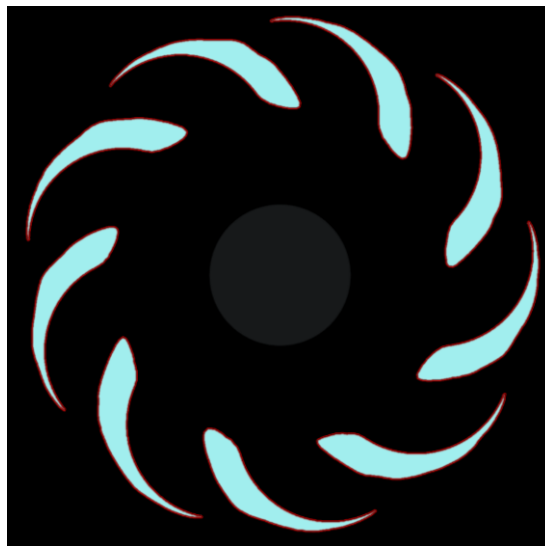
Figure B.2 - Binarized 0 velocity MATLAB output with overlay of detected white regions.
