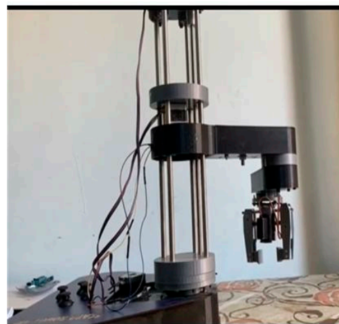
Figure 2. SCARA robot SolidWorks model design and its completed implementation.
