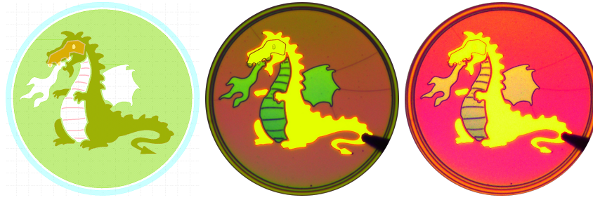
Figure 4.1: A test structure which illuminates when a current is applied. On the left is shown the mask layout, the right two figures show fabricated structures which illuminate when current is applied.
