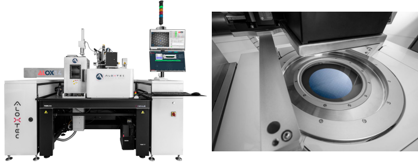
Figure 3.13: The Aloxtec conduction furnace used to perform the wet oxidation process on these VCSELs. The wafer is held by vacuum pressure against a heated chuck in the furnace. An infrared microscope image the sample during the processing.
