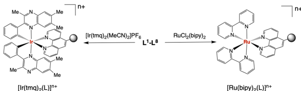
Scheme 3. Final Synthetic Step to the Different Ru(II) and Ir(III) Complexes
