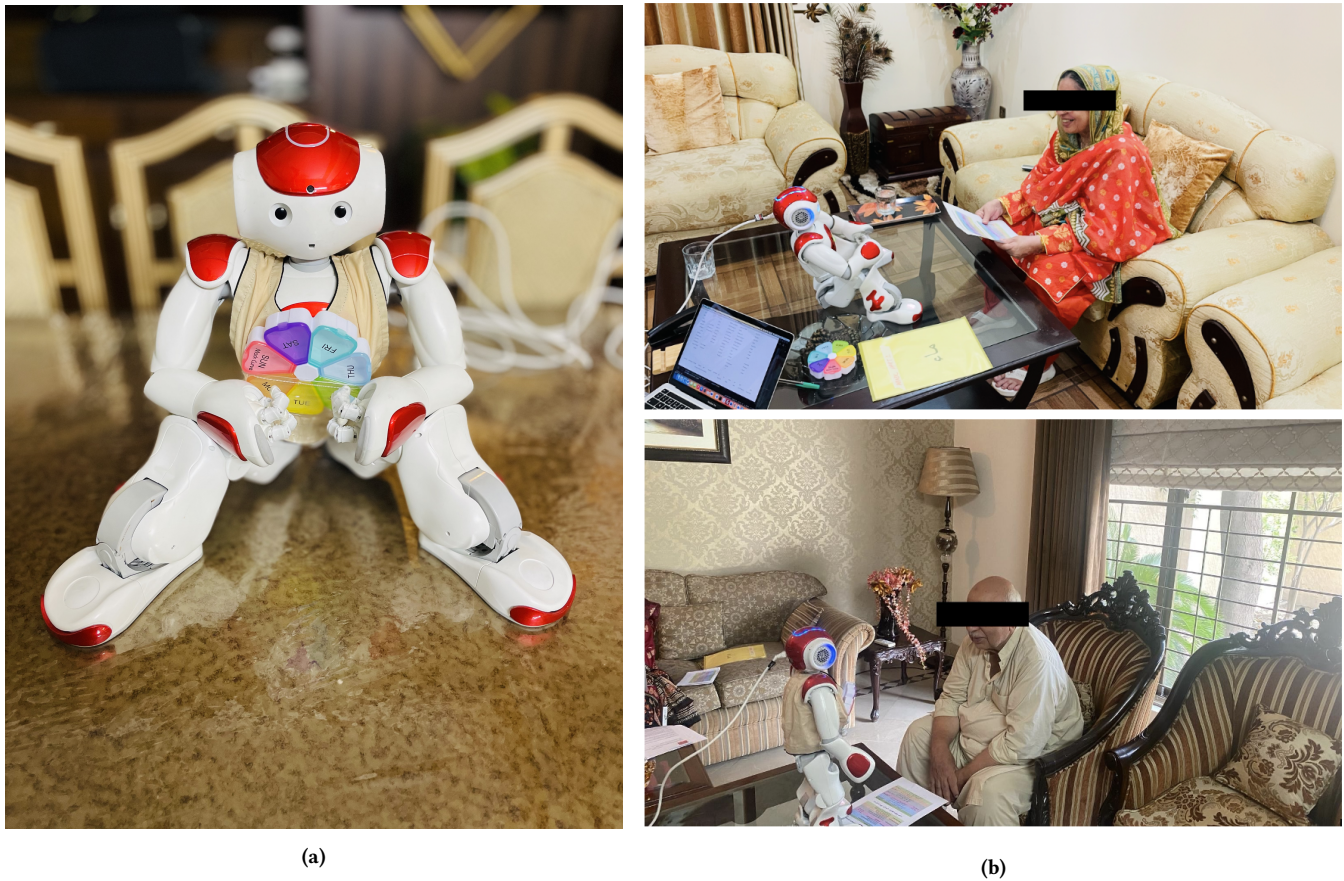
Figure 1: Left: Robot used during the study. A vest and a medication box were added to help older adults relate to it and remember their medications. Right: Examples of the study setup, with the robot interacting with the participants during the study.
