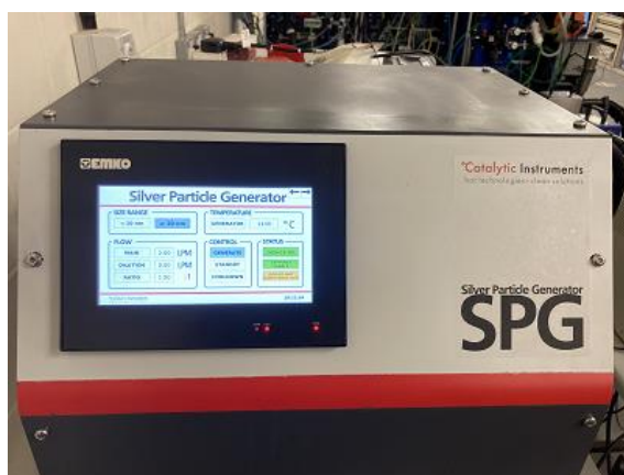
Figure 18: Photograph of Catalytic Instruments Silver Particle Generator (SPG) during trial
