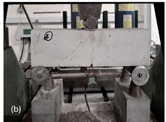
Fig. 2. Schematic representation of the three-point bending test setup on notched beam specimens (a), Experimental setup showing the test in progress with the loading applied at midspan and CMOD gauge installed at the notch (b).
