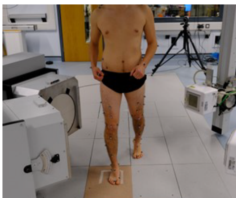
Figure 2-11 – Level gait equipment configuration with target area marked using masking tape.
