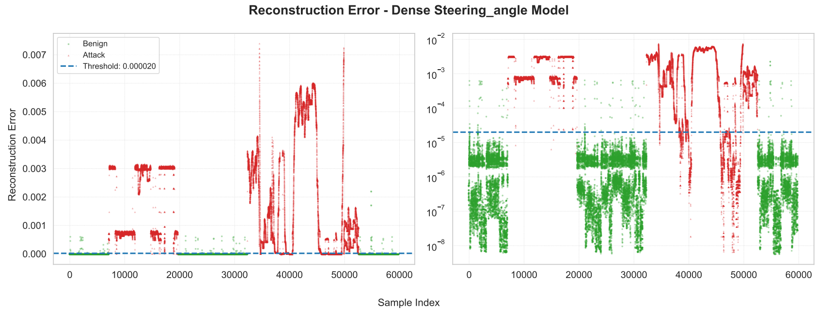
Fig. 5.17 Reconstruction loss of the fully-connected autoencoder's predictions on the steering angle test set.
