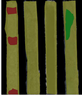
(b) Damage distribution on AR-4
