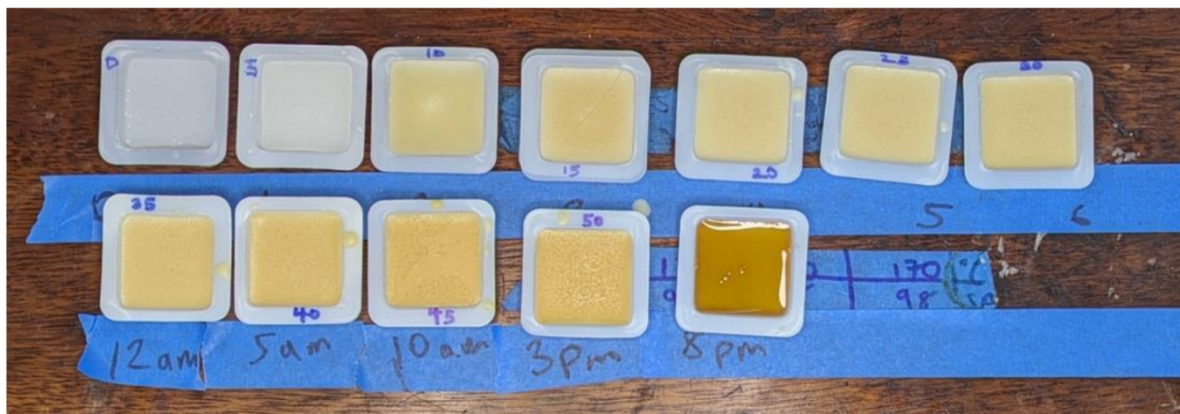
Supplementary Information 1: Picture of yellow/brown, waxy PES polymer from the transparent reactants over 60 hours.
