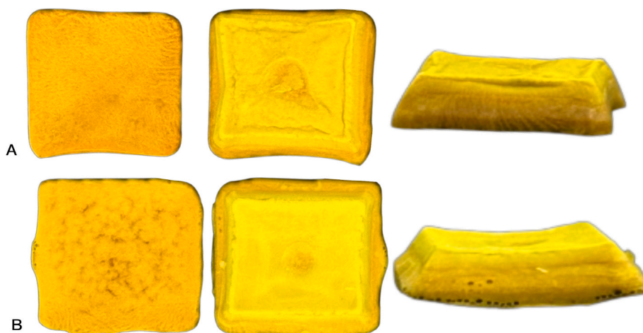
Fig. 4. Wafers seen from the top, bottom (backlayer) and side, containing: (A) CH and (B) CH:HPMC low , both with 4% w/w CUR-emulsion (1.45 mg CUR/wafer).
