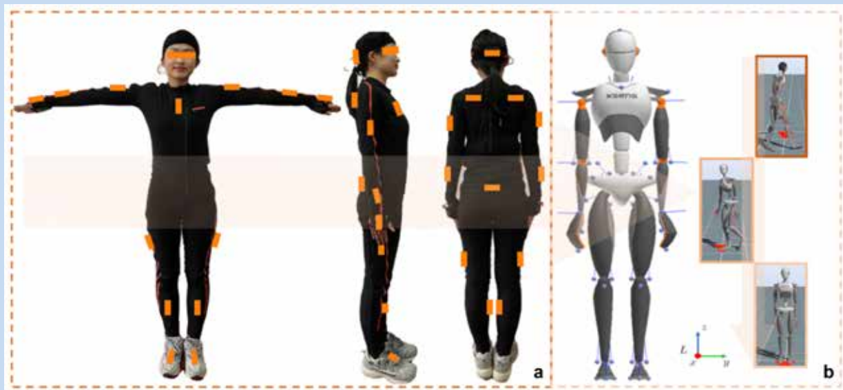
Figure 1. Sensor fixation and model construction. (a) Placement of IMUs of the MVN Link System on the body. (b) Process of model construction, including the establishment of joint coordinates essential for accurate kinematic analysis. IMU, inertial measurement unit.
