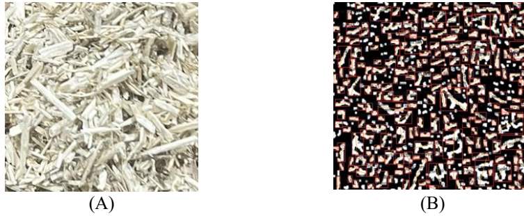
Figure 1. (A) Captured image of a hemp shiv sample (B) Binary analysis of the sample to identify the fibre size distribution.
