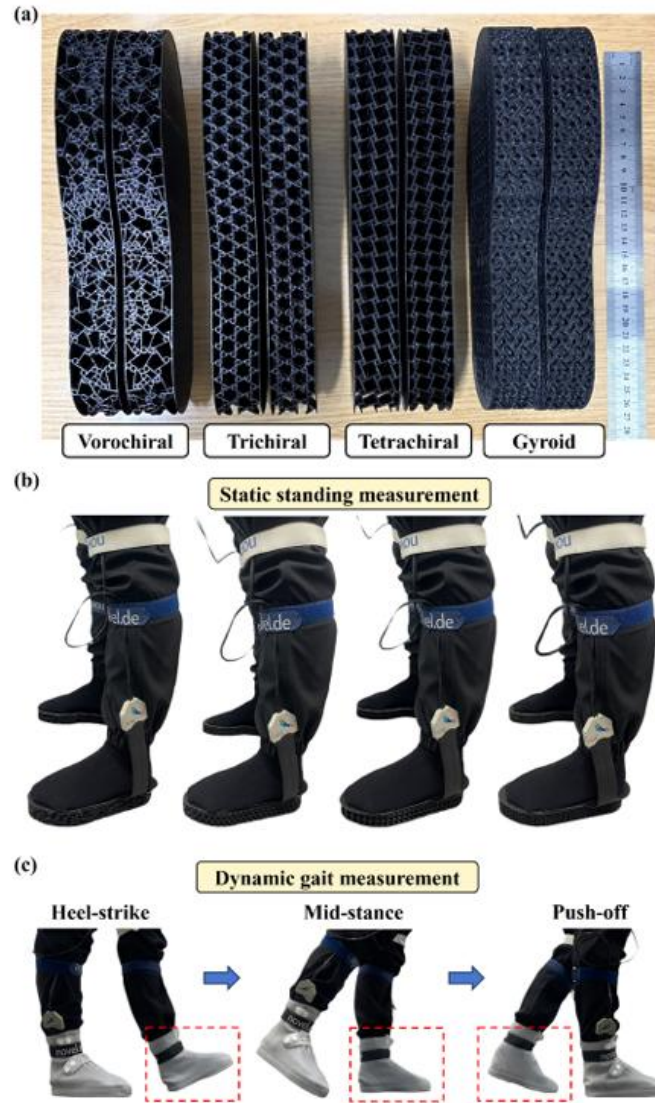
Fig. 10. Midsoles and measurements setups for static standing and gait analysis. (a) Four midsoles with Vorochiral, trichiral, tetrachiral, and Gyroid structures. (b) Static standing measurement setup. (c) Dynamic gait measurement setup.
