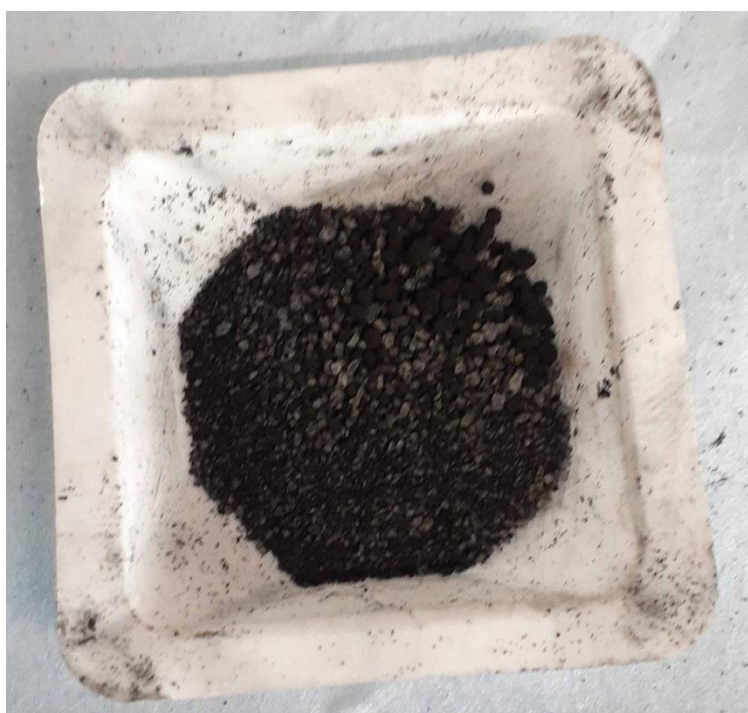
Figure 6.2 – Manually mixed magnetite and post-consumer HDPE powder
