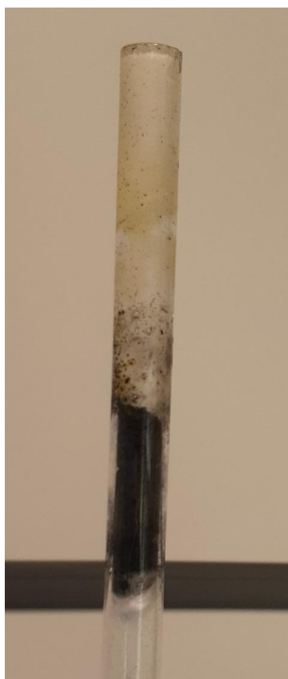
Figure 6.11 – Post-reaction tube showing waxy/liquid deposits on tube surface
