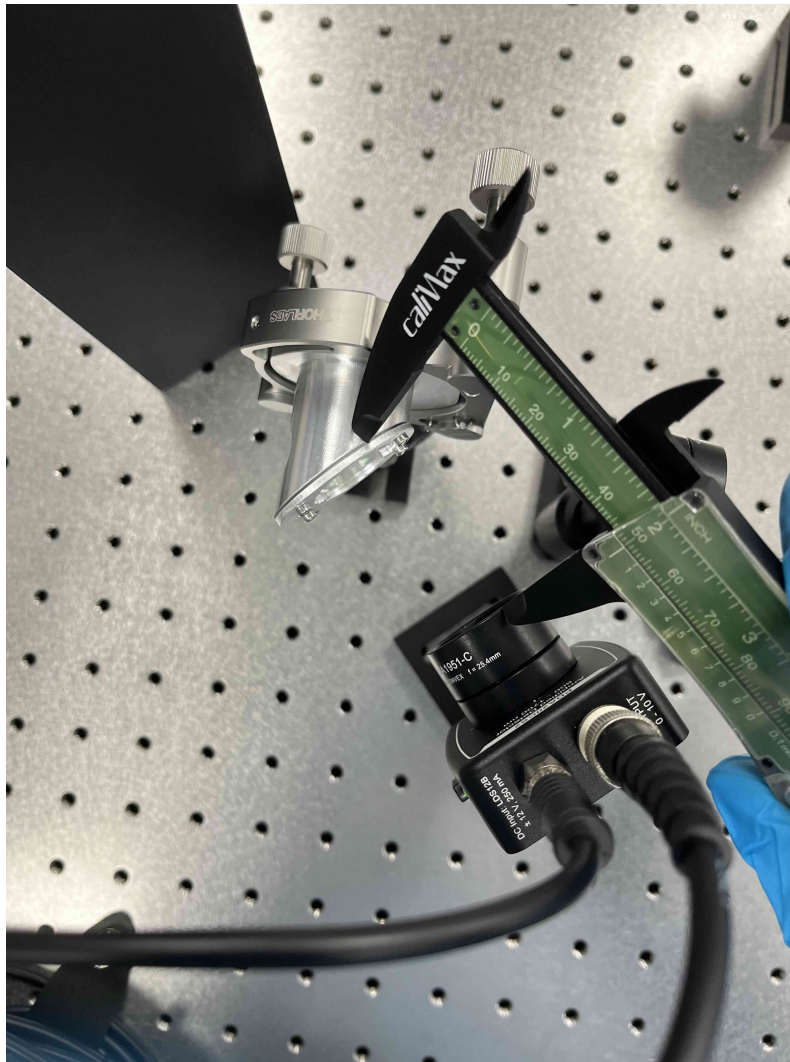
Figure 7.2. Optical setup for BS scatter power estimation. A beam block is used behind the BS mount to minimize stray scattered light. The measurement was performed with all ambient light sources in the room turned off.
