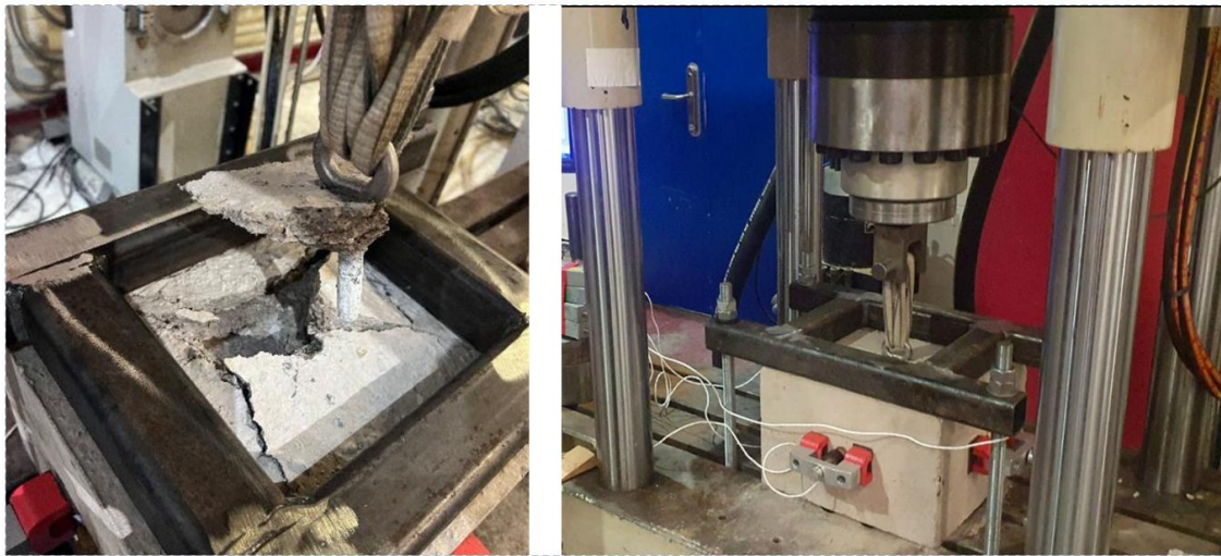
Fig. 3. Photos of the testing setup. An example of resin bolt failure (left), and an image showing the restraining method and sensor mounting method, along with the sling connection between the load machine and bolt.
