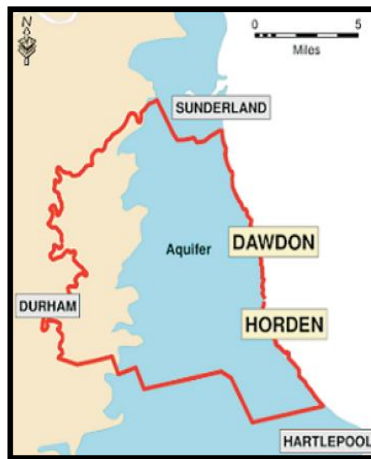
Figure 3-6: Area of East Durham aquifer protected by pumping at Dawdon and Horden 2
