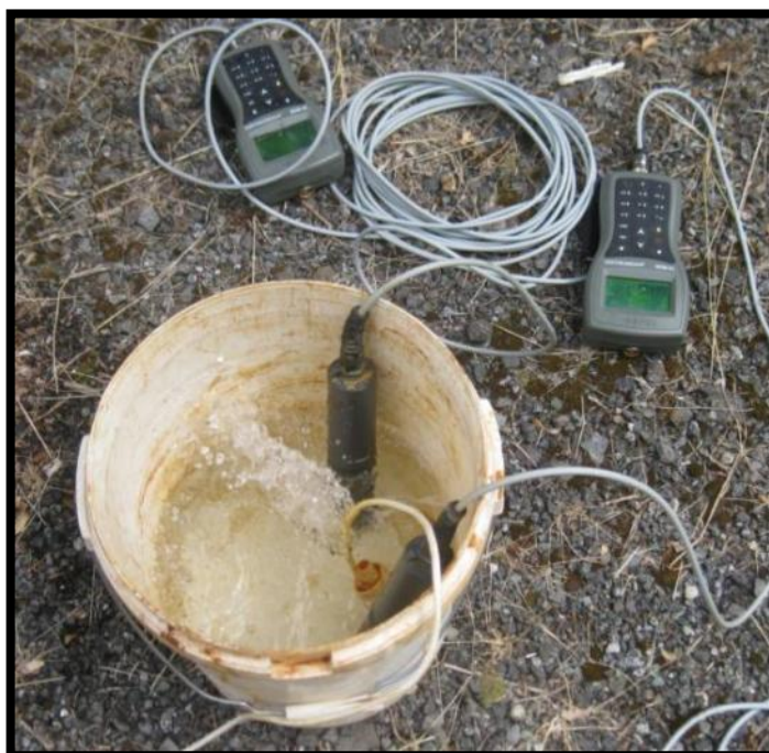
Figure 4-2 Experimental set up for homogeneous oxidation experiments
