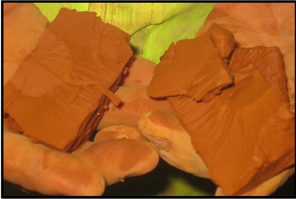
Figure 2-14 Dewatered sludge from filter press at Dawdon
