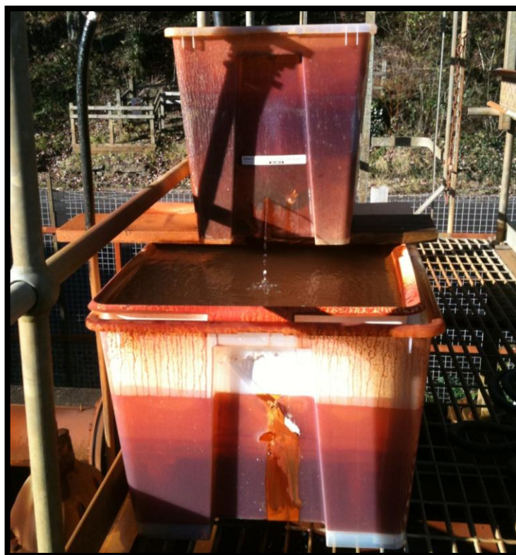
Figure 5-13: The continuous flow VFR after 10 days of operation showing ochreous deposits on all surfaces
