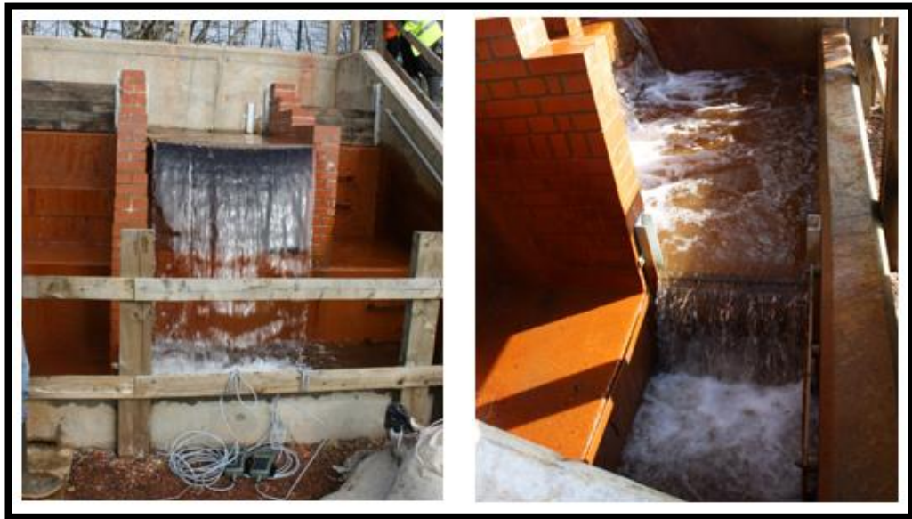
Figure 4-6 Configuration (a) single drop into plunge pool
