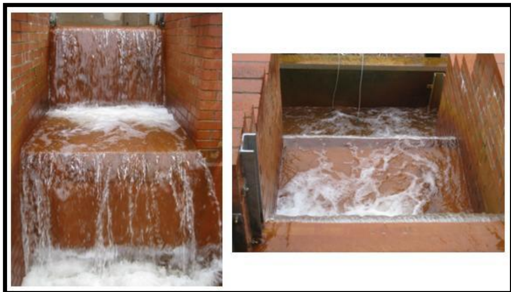
Figure 4-9 Configuration (d) two steps, weir board, water level in channel 37cm
