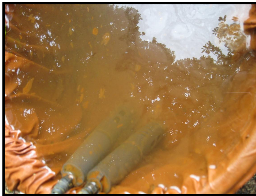
Figure 4-20 Logging pH measurements in the bucket VFR showing how solids settled leaving clearer water over time.
