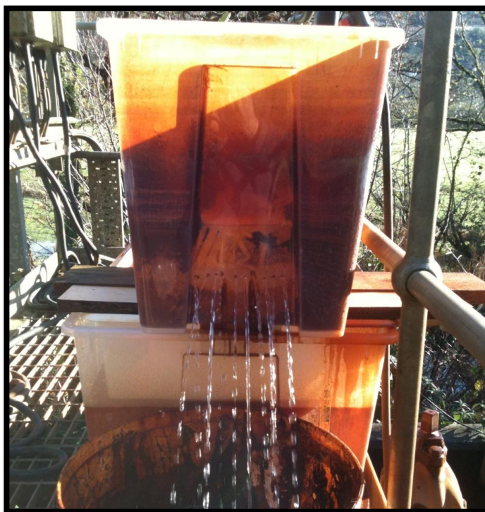
Figure 5-14: Flow rate regulation in the continuous flow VFR showing water flowing out of the back of the header tank to prevent overspill
