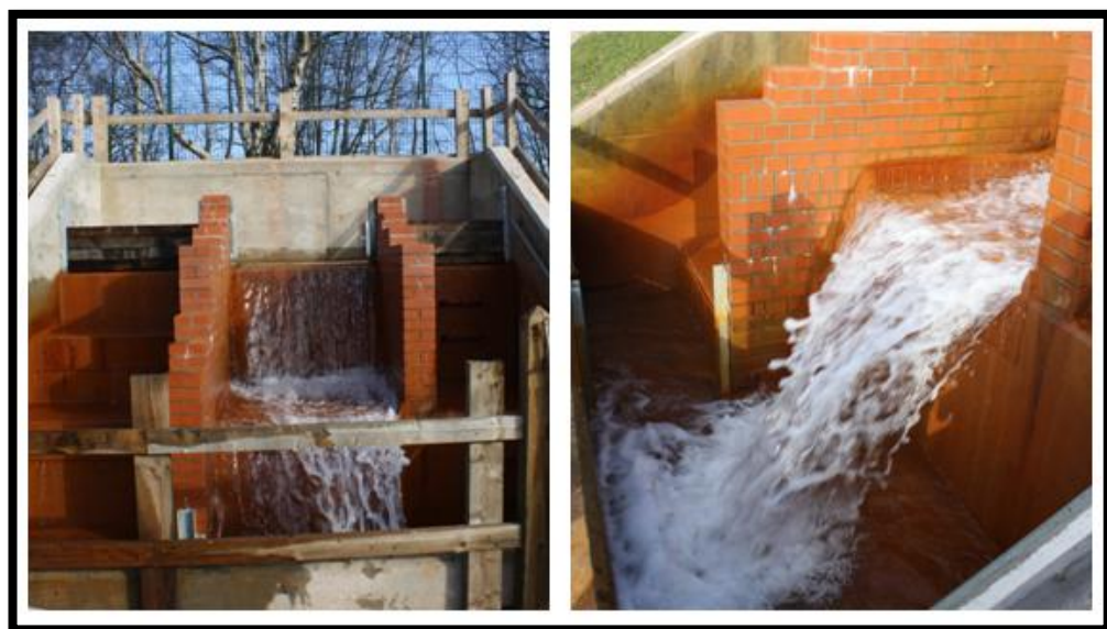
Figure 4-7 Configuration (b) two steps no weir boards
