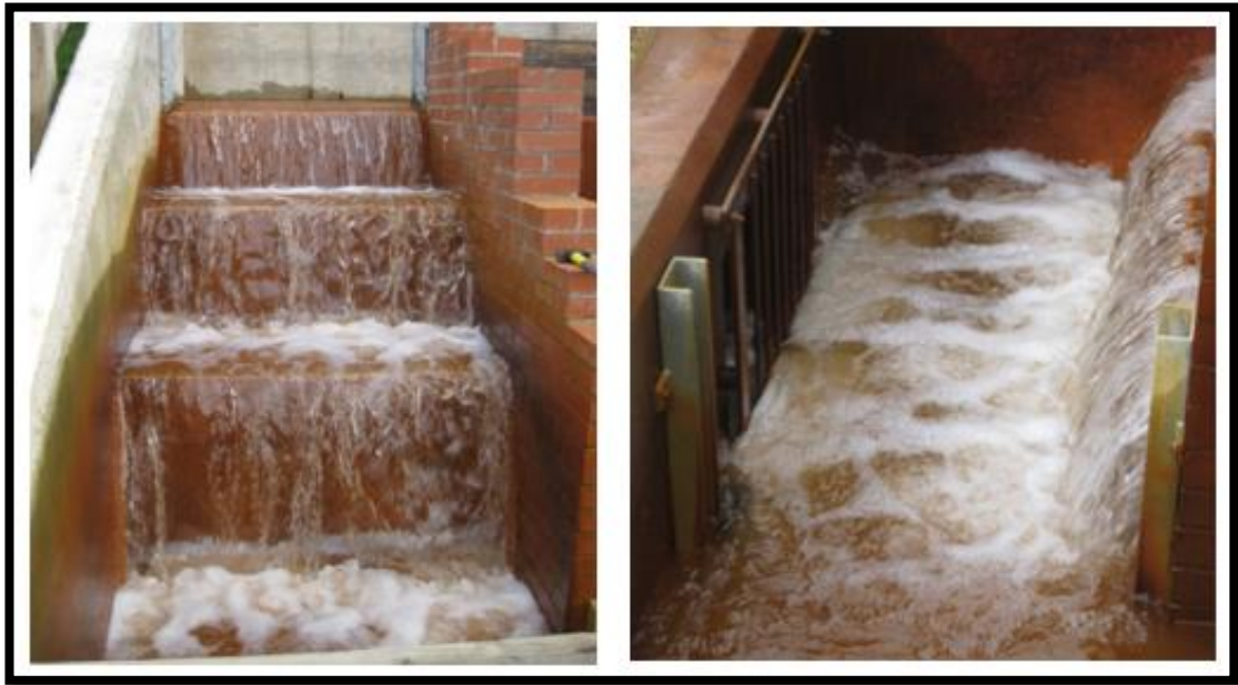
Figure 4-10 Configuration (e) three steps, weir boards, water level in channel 37cm
