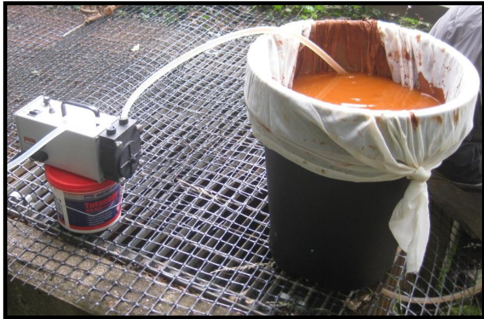
Figure 4-19 Bucket VFR being filled with peristaltic pump
