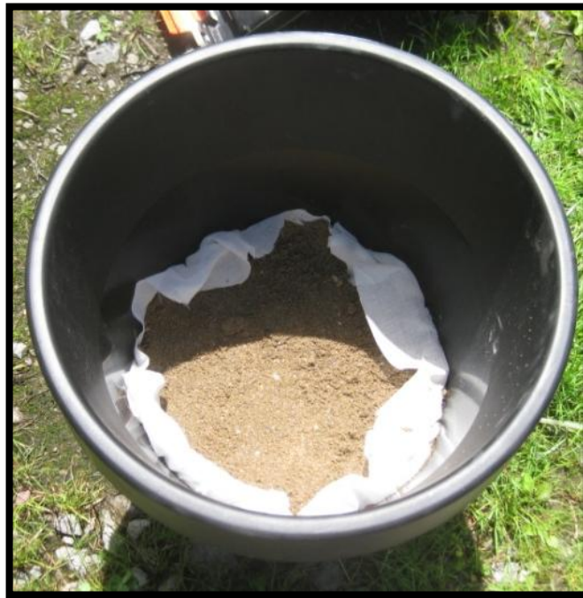
Figure 4-18 View of the bucket VFR with first muslin and sand layer
