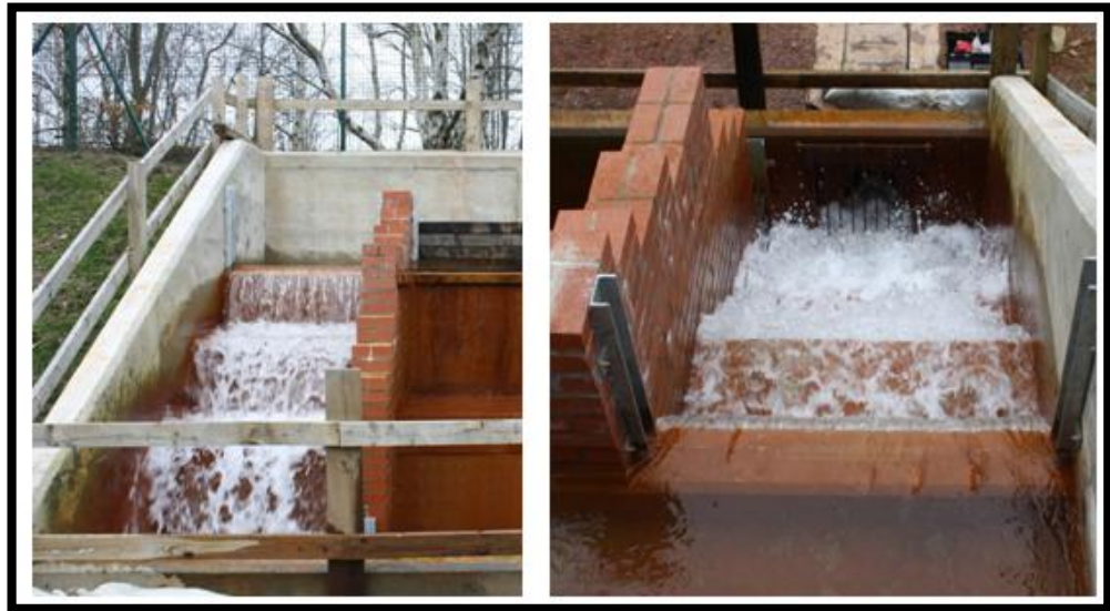
Figure 4-8 Configuration(c) three steps no weir boards
