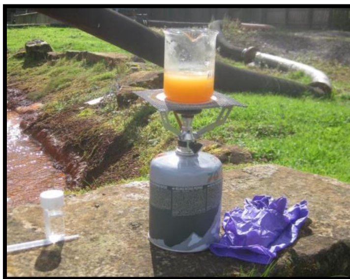
Figure 4-1 Experimental set up for hot peroxide titration
