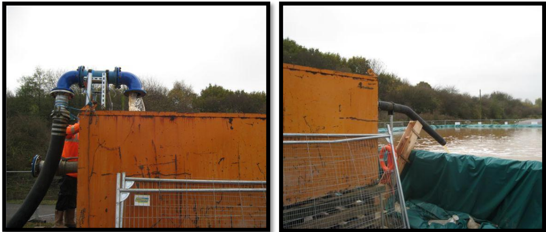
Figure 3-4: Premixing chamber for H_2O_2 and flocculent dosing at the Cadley Hill pumping trial
