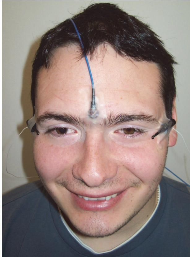
Figure 3.1.1: Participant prepared for ERG recording with DTL fibre holders adjacent to each eye (active and reference electrodes) and a skin (earth) electrode attached to the forehead.
