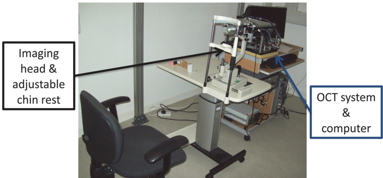
Figure 5.1.1: The 1060 nm OCT system; adjustable table, chin rest, imaging head and OCT system shown.
