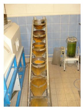
Figure 5.10 Photograph of the vibrating siever used to separate the pellets into the desired size fractions.
