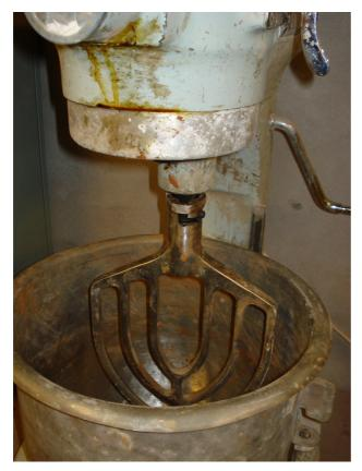
Figure 5.8 Photograph of the dough type mixer used for the mixing of cement and the sludge from Horden minewater treatment plant
