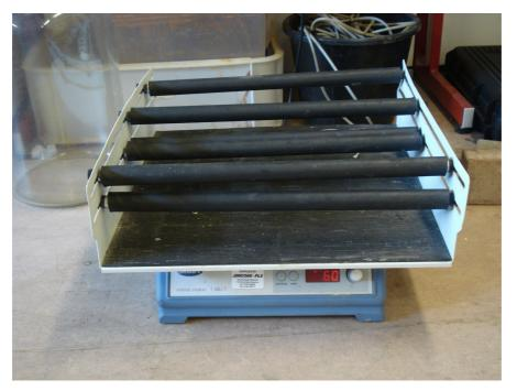
Figure 5.7 Photograph of the shaker table used in the batch experiments
