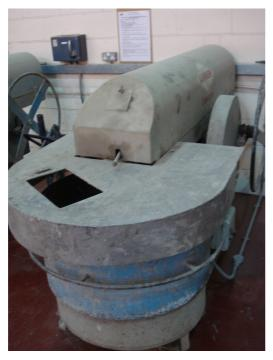
Figure 5.18 Linear drum mixer used for column pellet production
