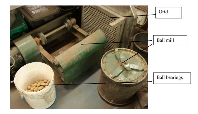
Figure 5.19 Ball mill used to crush material down to suitably sized pellets
