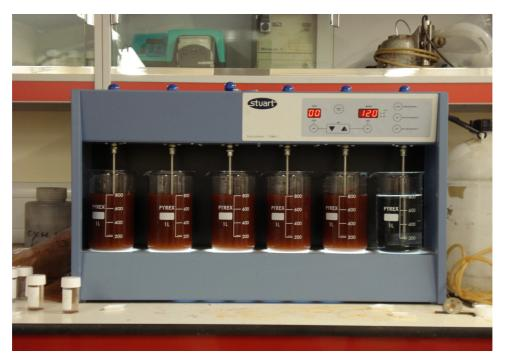
Figure 5.6 Photograph of the flocculator used for the kinetic tests on the solids from Horden
