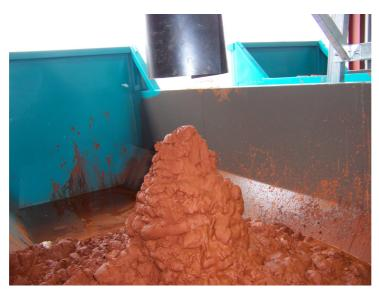
Figure 5.1 Photograph showing the treated sludge form Horden minewater treatment plant as it is discharged from the centrifuge at the treatment plant.
