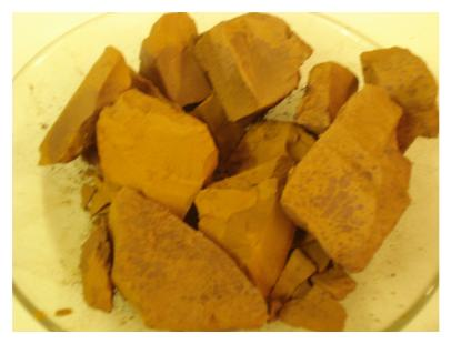
Figure 5.4 Photograph of the solids from the Dawdon minewater treatment plant
