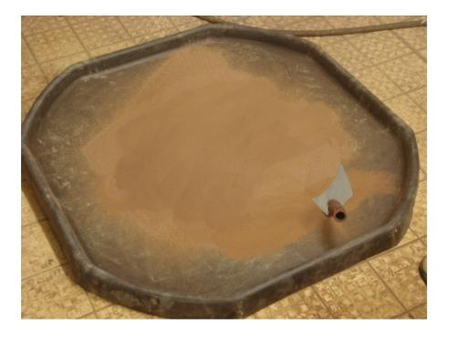
Figure 5.20 Blending of the various pellet sizes
