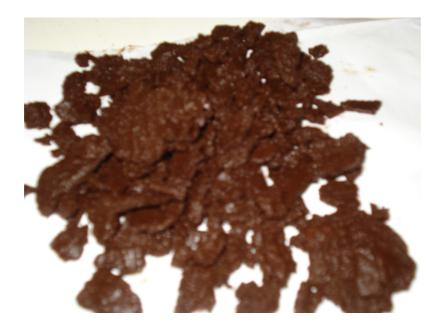
Figure 5.2 Photograph showing the filter cake from a water treatment plant
