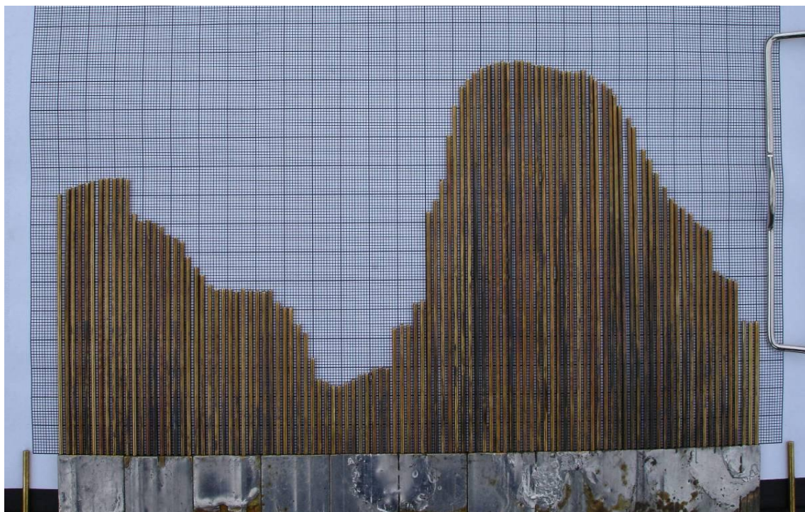
Figure 2. Profiler and example of a river bed profile used to assess surface complexity and area for 0.25 x 0.25 m sampling locations.
