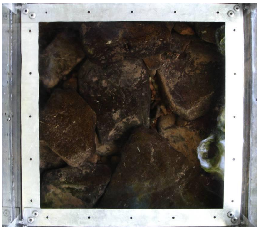
Figure 3. Sampling frame (0.25 x 0.25 m) showing the location of holes for positioning the profiler.
