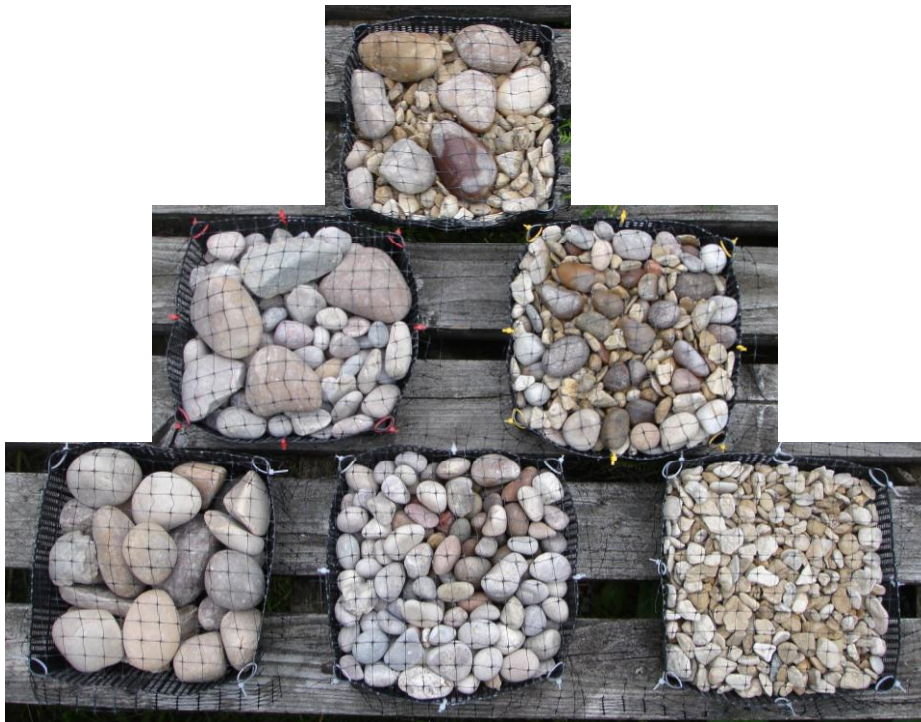
Figure 2. Examples of experimental baskets filled with cobbles, pebbles, gravel and 50:50 mixtures.
