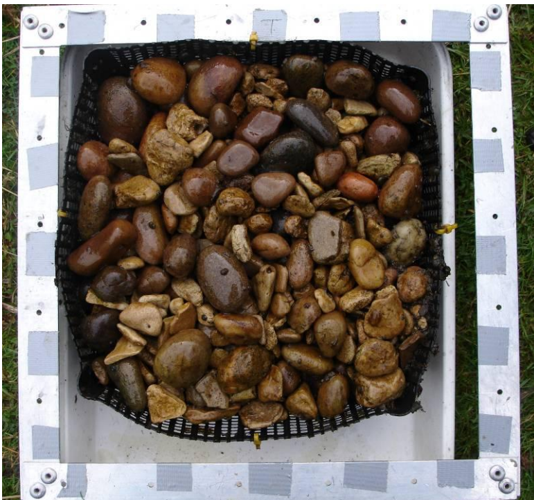
Figure 4. Sampling frame (0.25 x 0.25 m) showing the location of holes for positioning the profiler.
