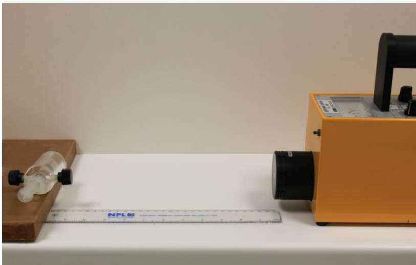
Fig. 6.6 Measurement taken from the edge of the syringe to assess true effect of shield.
