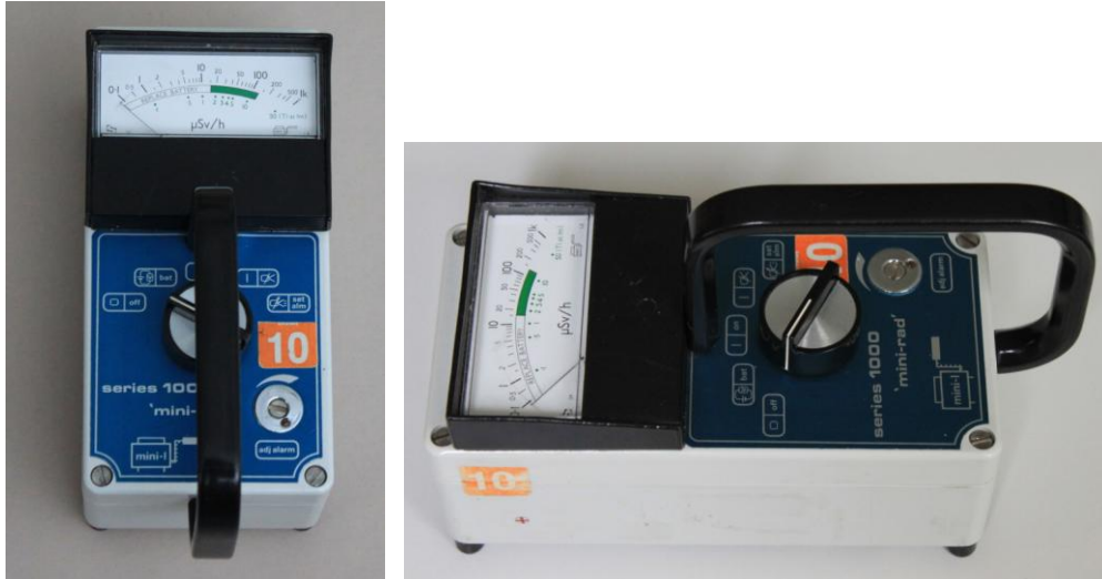
Fig. 6.1 Mini-Rad Series 1000 radiation dose rate monitor.
