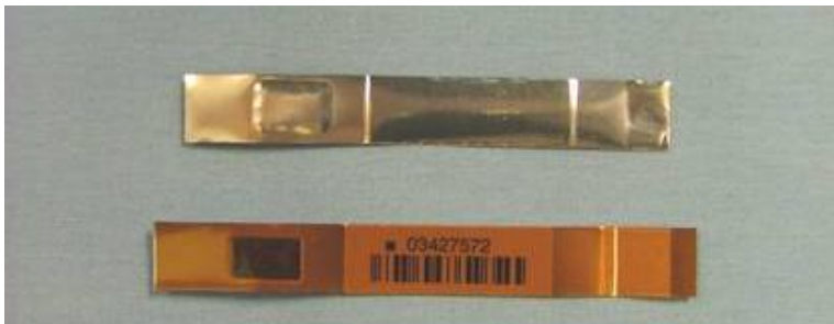
Fig. 5.1 NE-Technology LiF-7 powder TLD
