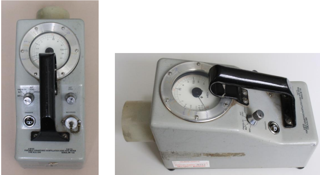
Fig. 6.3 NIS 295B portable logarithmic scintillation dose rate meter monitor.
