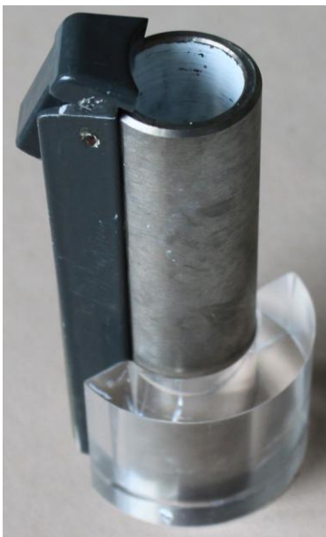
Fig. 5.9 1cm curved Perspex providing a snug fit to the shield.
