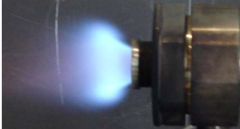
Figure 6.5: Attached flame of coke oven gas \dot{m}_f = 0.725\text{g/s} , \dot{m}_a = 10\text{g/s} , \phi = 1.1 (just before flashback) for the swirl burner S=1.04
