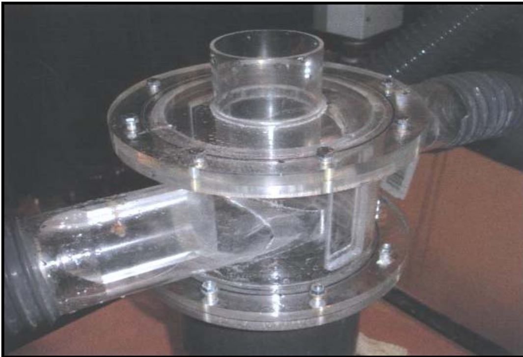
Figure 4.1: The Perspex swirl generator
