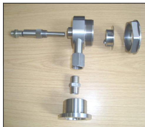
Fig. 1. Exploded view of swirl burner.
