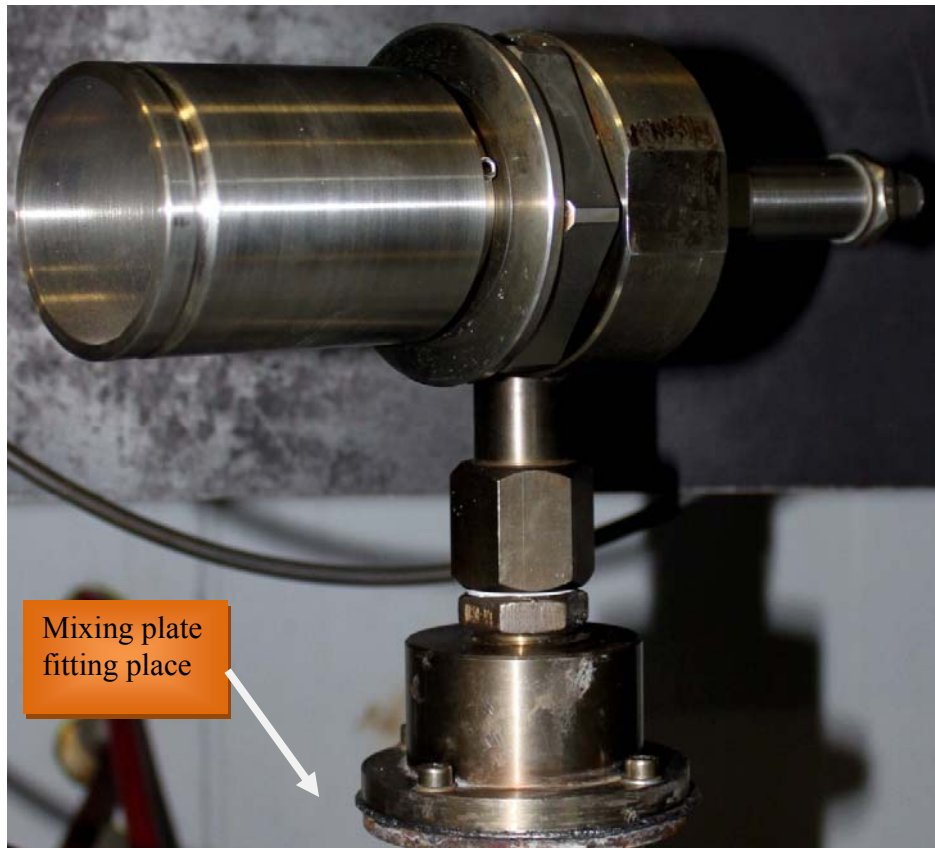
Figure 5.11 Swirl burner fitted with open cylindrical confinement
