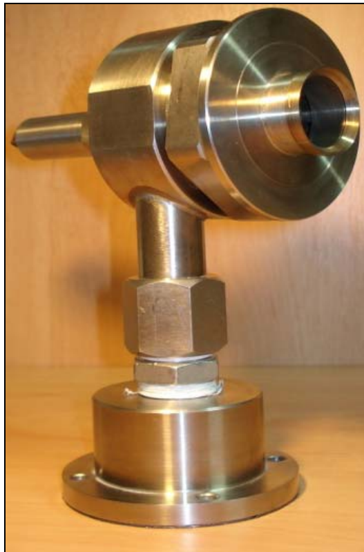
Figure 5.10: The assembled swirl burner S=1.04
