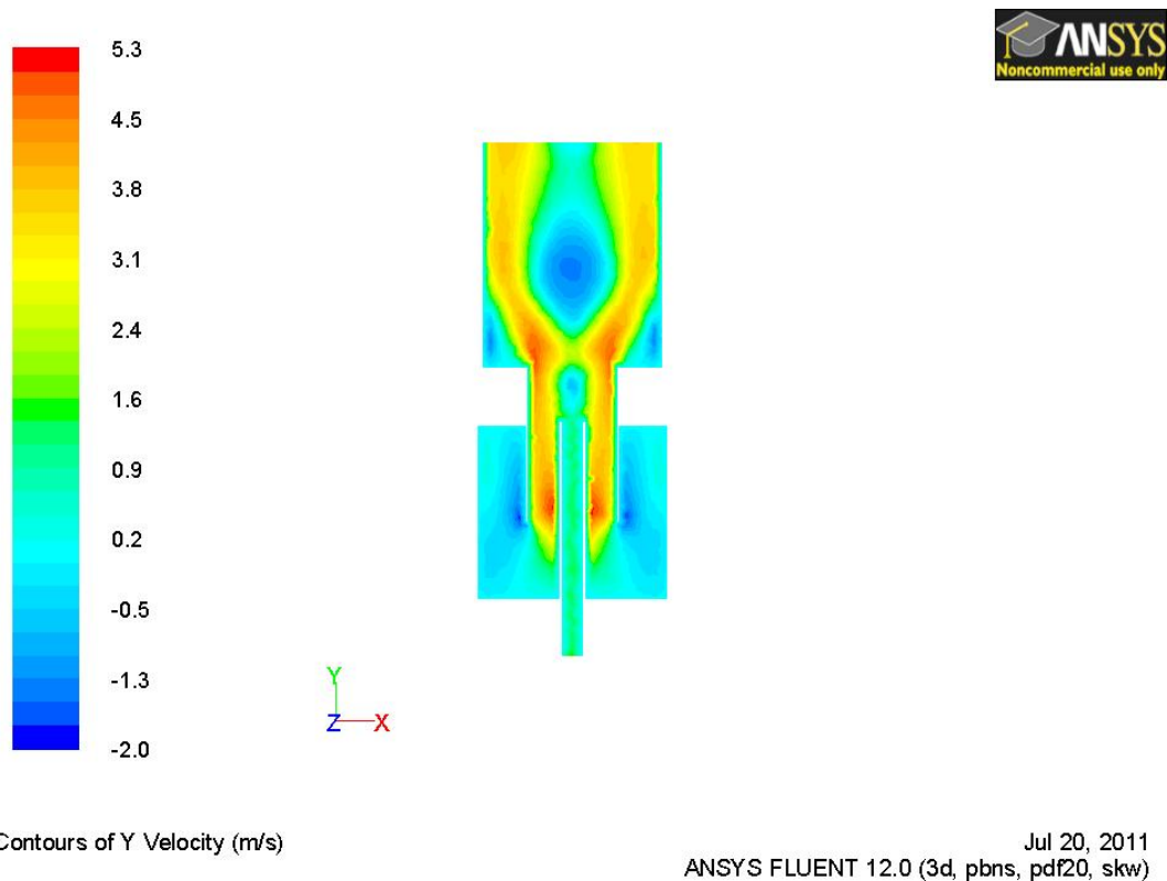
Figure 2.2 Velocity contours with combustion in a swirl burner
