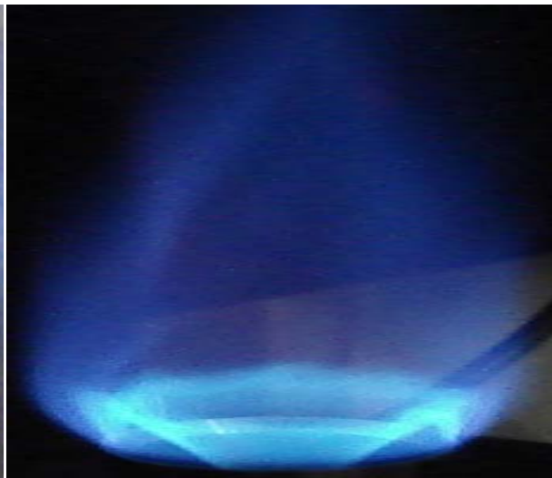
Figure 6.2.b: Photo of flame just before flashback through outer wall boundary layer, S_B=1.04
