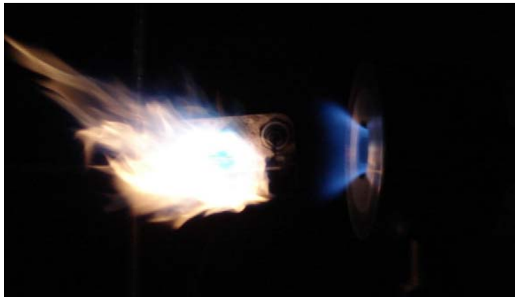
Figure 6.8: Rich hydrogen flame \dot{m}_f = 0.5 \text{ g/s} , \dot{m}_a = 11 \text{ g/s} , \phi = 1.5545 for the swirl burner at S=1.47 . Note use of propane torch again.
