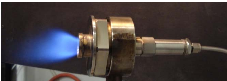
c: S_C=0.8 \dot{m}_f = 1.0 g/s, \dot{m}_a = 17 g/s \phi = 1.012
