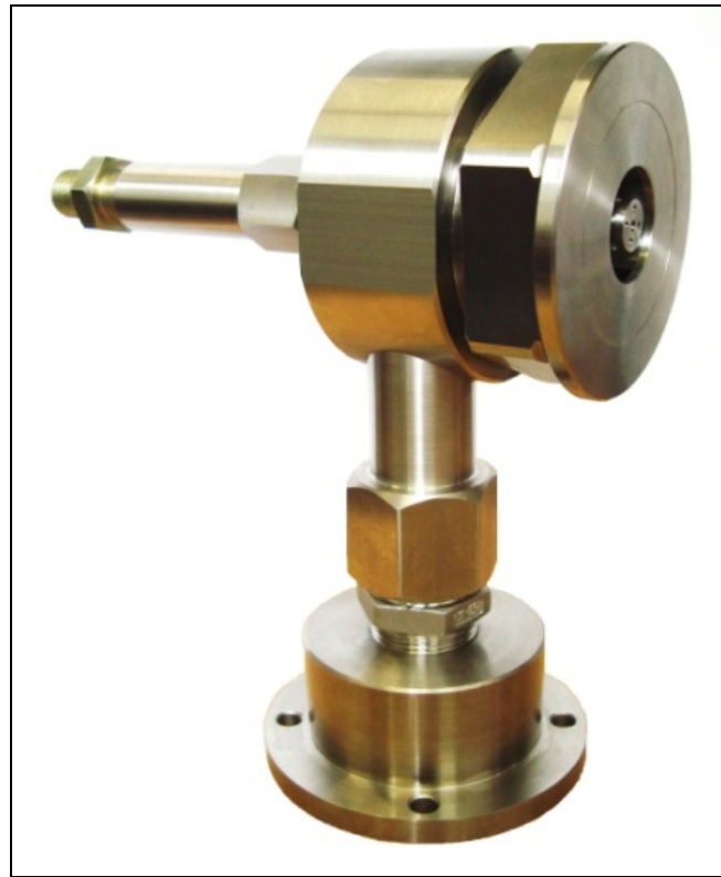
Figure 5.2: The assembled swirl burner S=1.47
