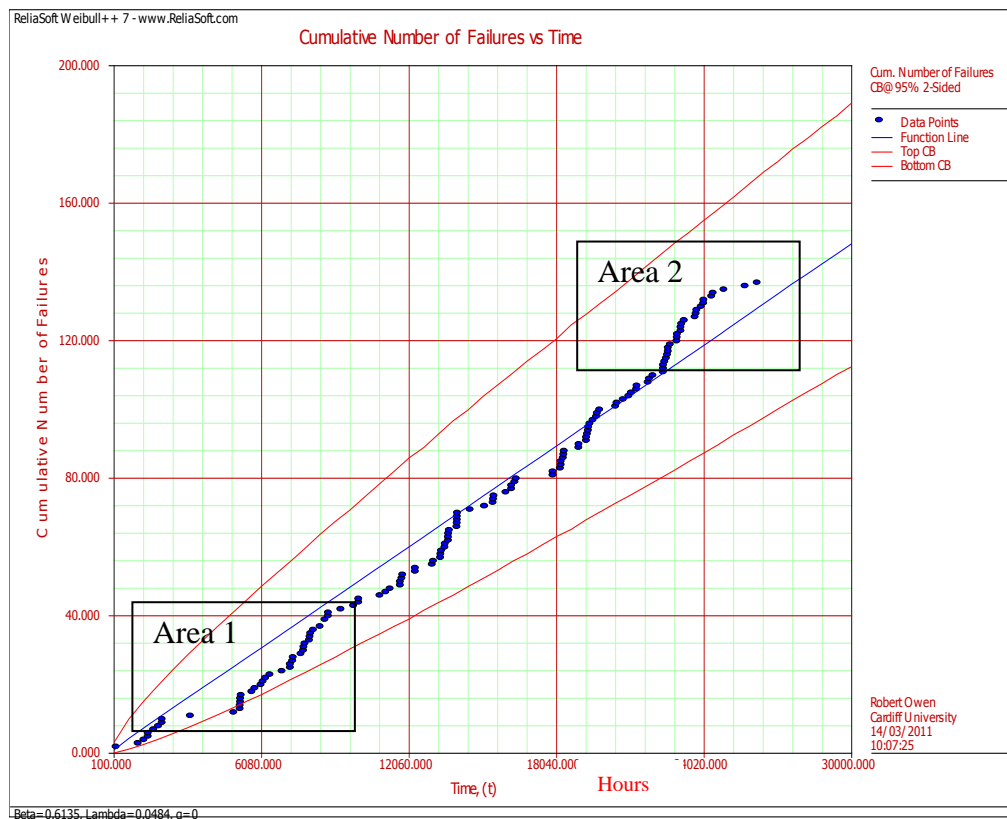
Figure 5-4 Weibull ++ RDA plot of Coiler 5 data set, Cumulative Failures versus Time (Hours)
