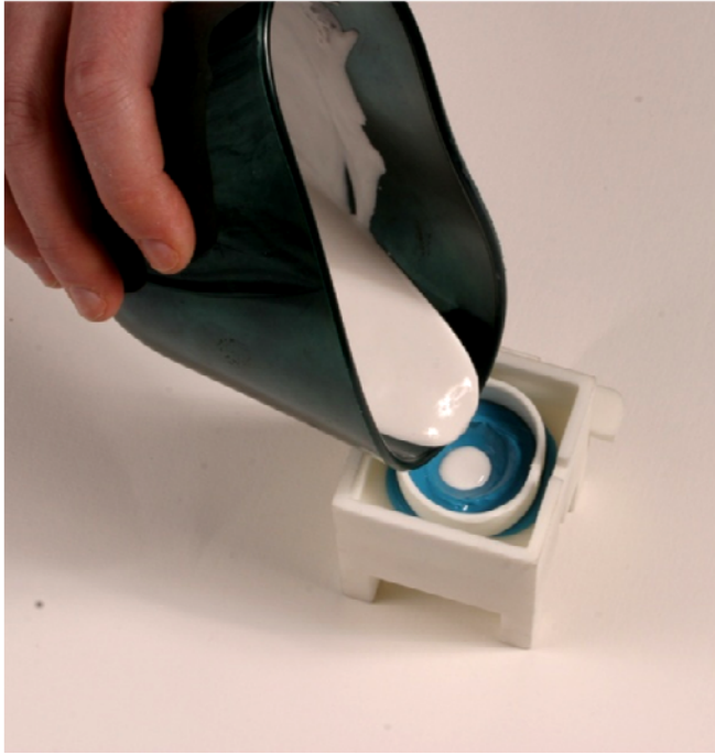
Figure 8.3: Photograph showing wet plaster being poured into the die cavity (courtesy of Benjamin Jones).
