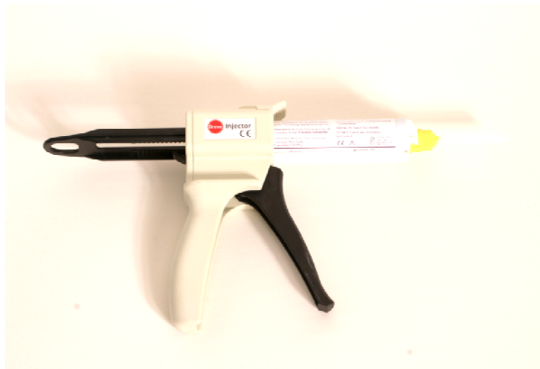
Figure 5.2: Injector DS 50 (Dreve Otoplastik GmbH, Germany), with a Tresident dual cartridge and mixing canula.
