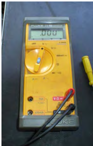
Figure 3.8. Voltmeter to read pressure gauge from orifice pressure gauge
