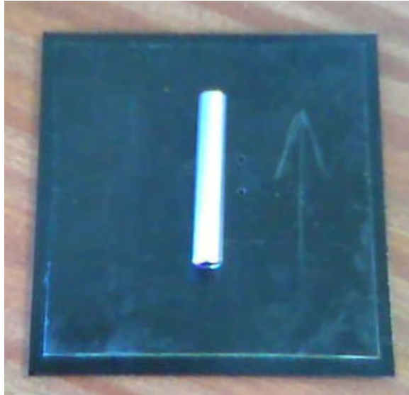
Figure 4.11. Sheath to protect air temperature measurement thermocouple
