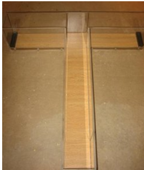
Figure 3.2 T-maze apparatus, showing maze construction and recessed wells.
