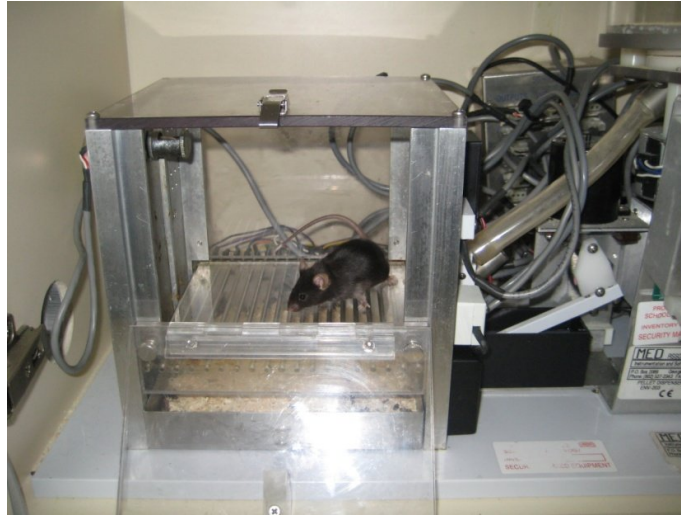
Figure 4.26 Mouse operant chamber and set-up used for biconditional discrimination, Stroop task and reversal learning experiments. Photograph depicts Context 2 (smooth flooring) with transparent polycarbonate sheet used in 8 of the 16 chambers. Context 1 (bar flooring), used in the remaining 8 chambers, was identical but without the transparent polycarbonate sheet on the floor.
