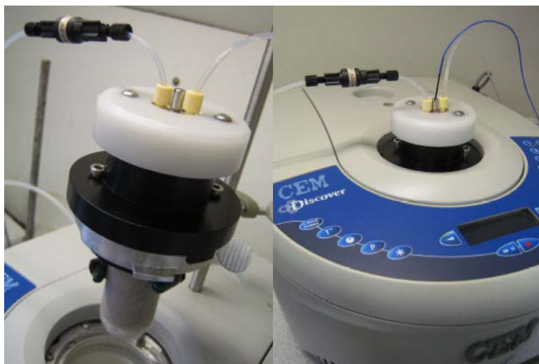
Figure 16. 80 mL flow cell setup 2
