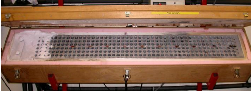
Figure 2.13 One of three temperature gradient system used for incubating pure methanogen cultures. Manufactured at the Earth Science department workshops, University of Bristol. Based on the design of Isaksen et al. (1994).
