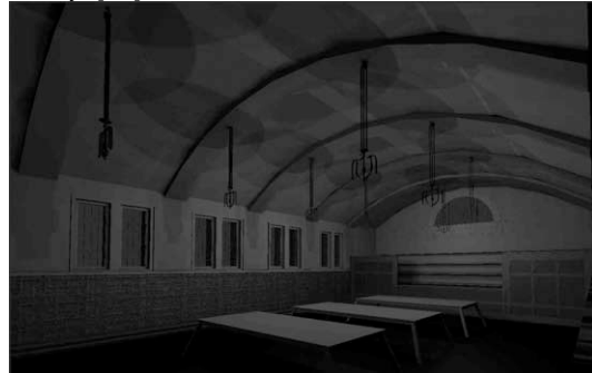
Fig. 7 Ray traced model illustrating artificial illumination of Reference Room (NB light sources not depicted)
