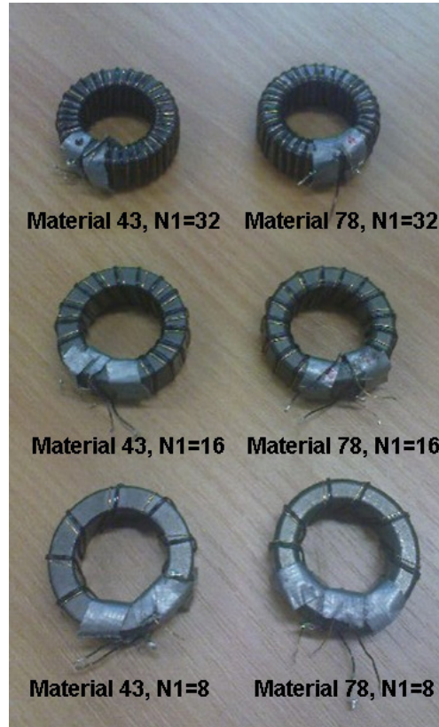
Figure 7.7: RF broadband transformers for two types of material with different number of turns on the core windings.
