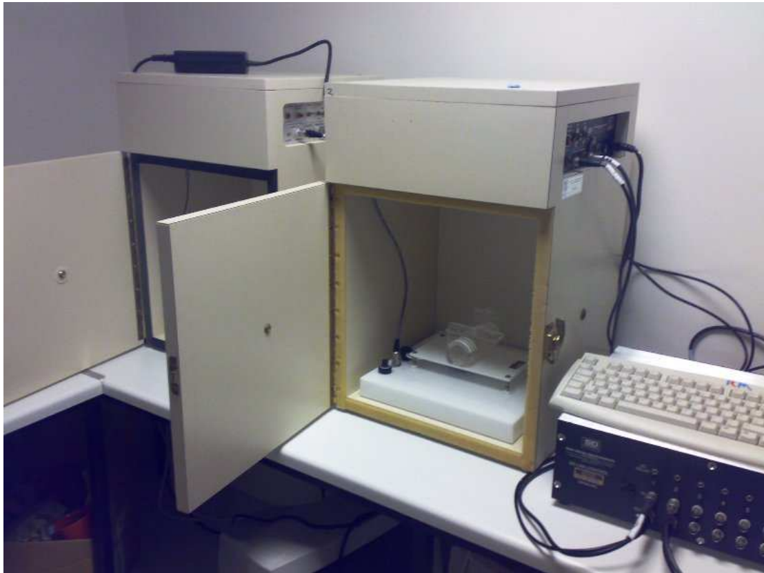
Figure 5. The startle apparatus used in this study. The picture shows two chambers connected to the computer, which save the data as Excel files.
