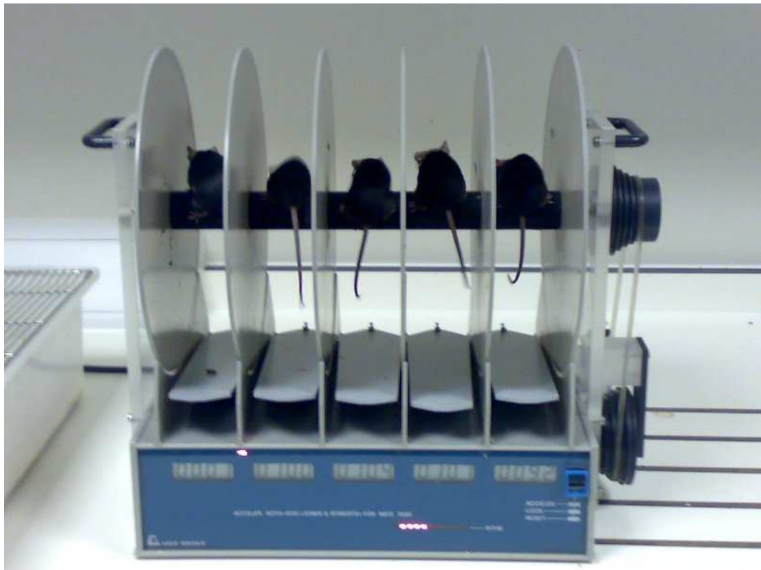
Figure 8. Mice rota-rod test apparatus (UGO BASILE COMERIO (VA) - ITALY) used to analyse the mice motor coordination and balance performance.
