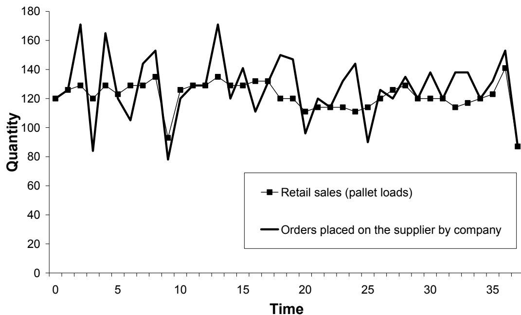
Figure 1. Bullwhip in the Real World ~ Substantial Demand Amplification Observed in the UK Retail Sector (Source: Jones, Hines and Rich, 1997)
