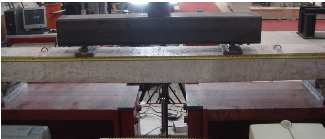
Figure 4.9b. Photo of flexural beam experiment
