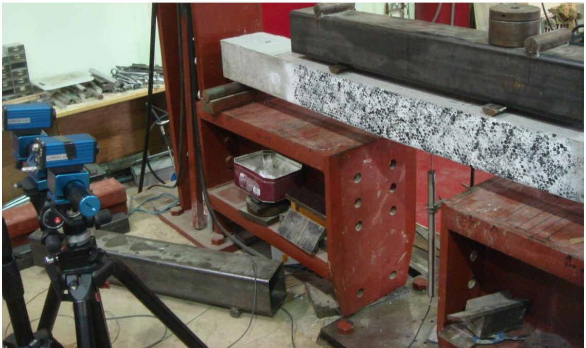
Figure 4.11c. Specimen being monitored by DIC camera system
