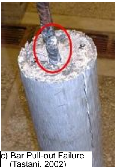
Figure 4.1. Four general types of failure in bond tests
