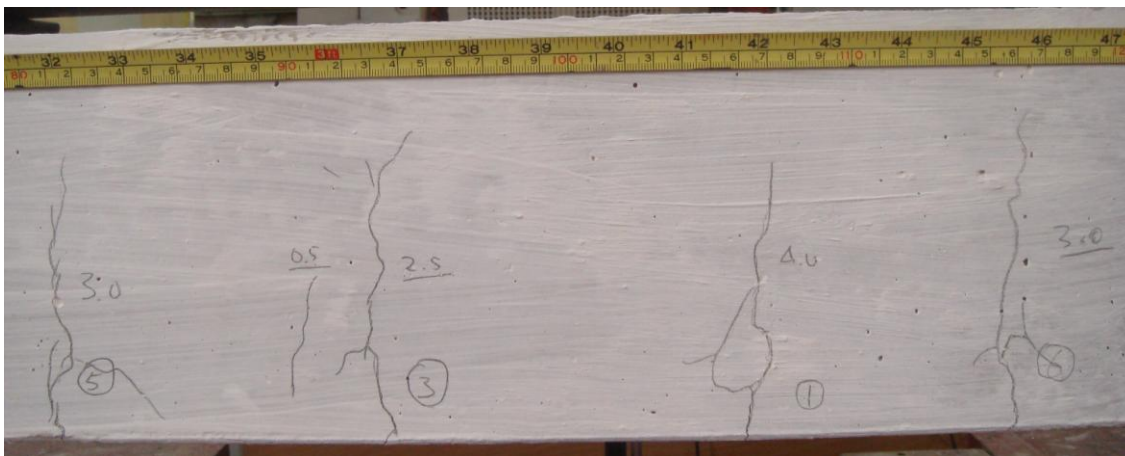
Figure 5.10. Cracked Celsa Beam
