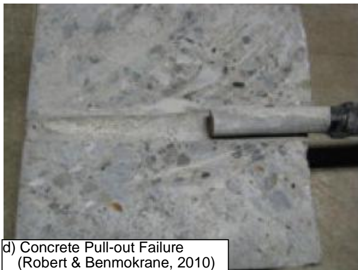
Figure 4.1. Four general types of failure in bond tests
