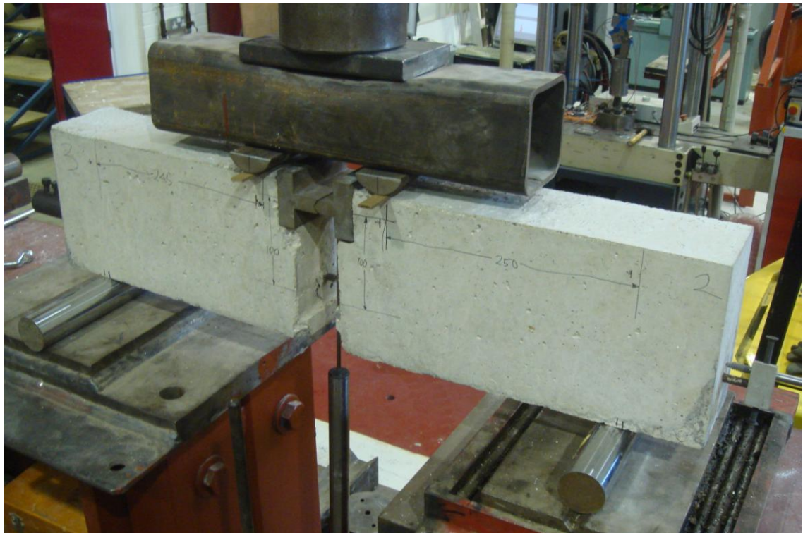
Figure 4.8b. Photo of bond beam experiment
