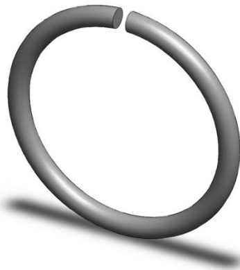
Figure 5.3: Split-ring resonator formed from a single piece of curved wire. This geometry is similar to those seen in Figure 2.8, including having a capacitive region located in the loop-gap and an inductive region opposite the loop-gap. The single wire approach is simpler to fabricate and less lossy than the planar implementation (Figure 2.8 a ), but demonstrates reduced electric field confinement in comparison with Figure 2.8 b .
