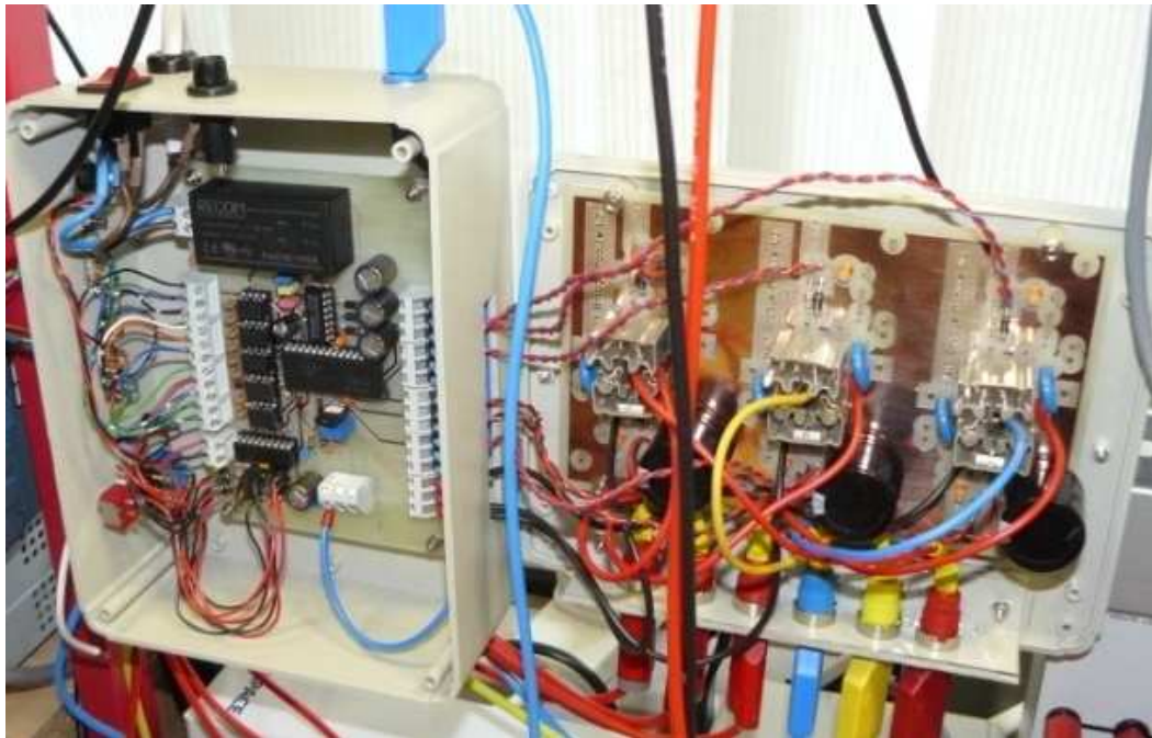
Figure 4.5 – Gate driver board (left) and 6 pulse MOSFET converter (right) forming one half of the back to back bridges, developed by the candidate and constructed at Cardiff University.
