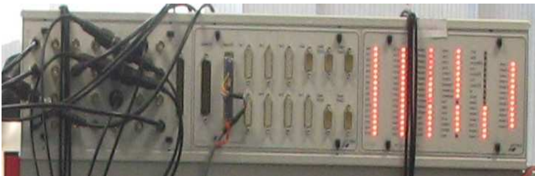
Figure 4.8 – Breakout panel for connection of sensors and digital I/O, including status LEDs for the digital I/O.
