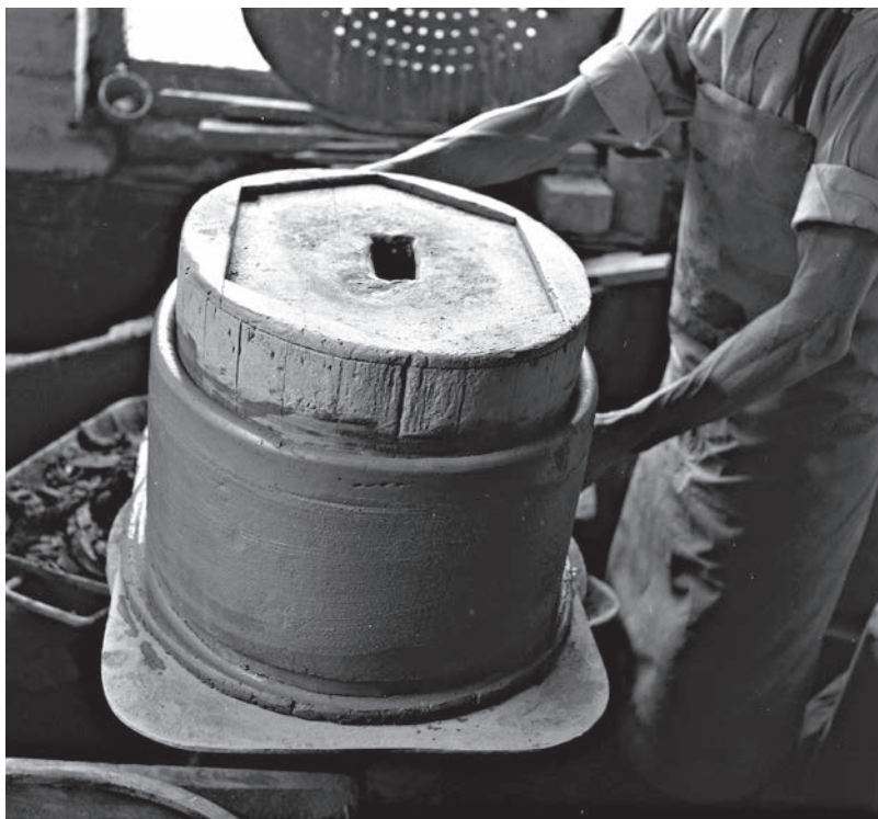
Plate 5.6. Mr. Fred Boulton has placed the drum covered in side-marl onto a ready knocked bottom on the wheelie. The hand-hole in the top of the drum is clearly visible. Photographed at the Burgess and Leigh Factory, Middleport 1964. (Photo by and reproduced courtesy of Mr. Donald Morris).
