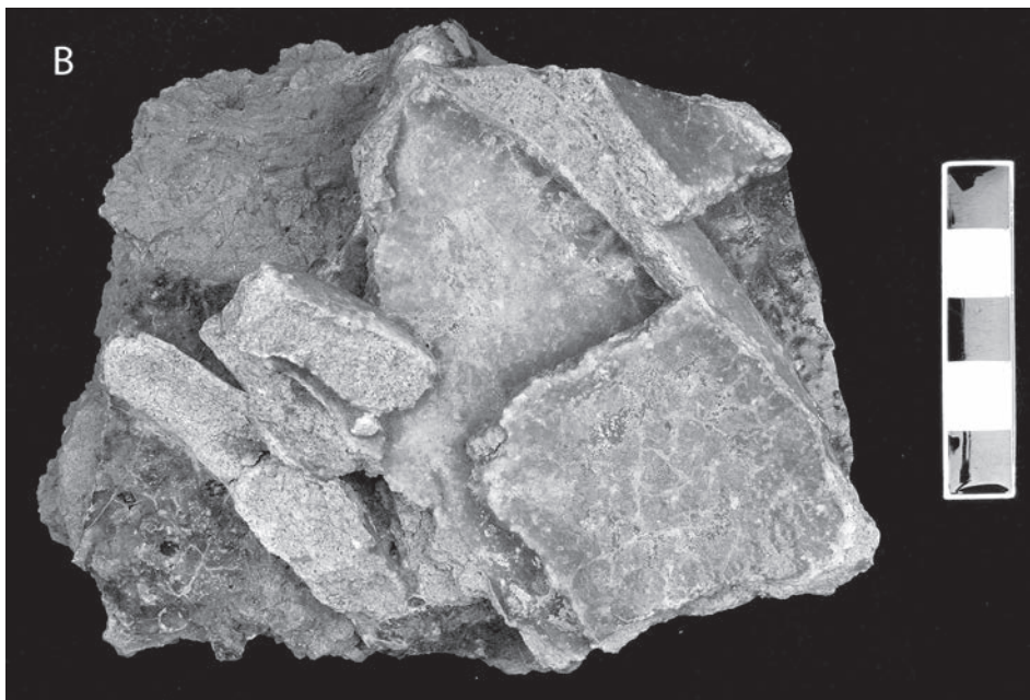
Plate 7.3. (A) Cross section showing a faience vessel (F-2025) of type T6.1a adhering to the base of a saggar. The thick layer of dark glaze can clearly be seen over the saggar base cementing the faience to it. (B) Fragments of faience vessel (F-129) of type T6.1a adhering to the base of a saggar. (Photos: P.T. Nicholson).
