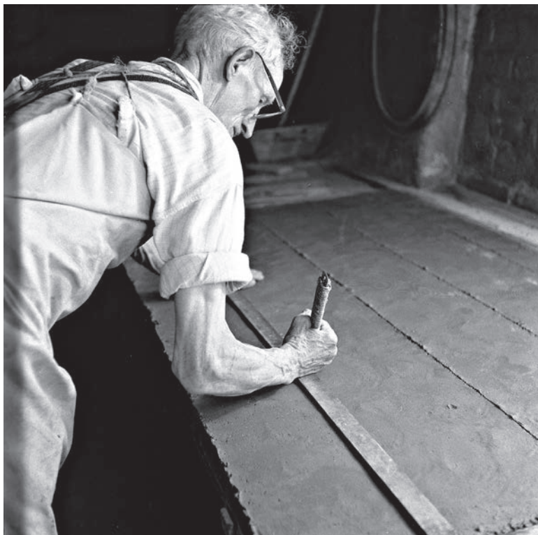
Plate 5.4. Mr. Fred Boulton using a wooden straight edge – 'rule' – and blade to cut strips of side-marl to the appropriate width ready to be rolled onto a wooden drum. Photographed at the Burgess and Leigh Factory, Middleport 1964. (Photo by and reproduced courtesy of Mr. Donald Morris).
