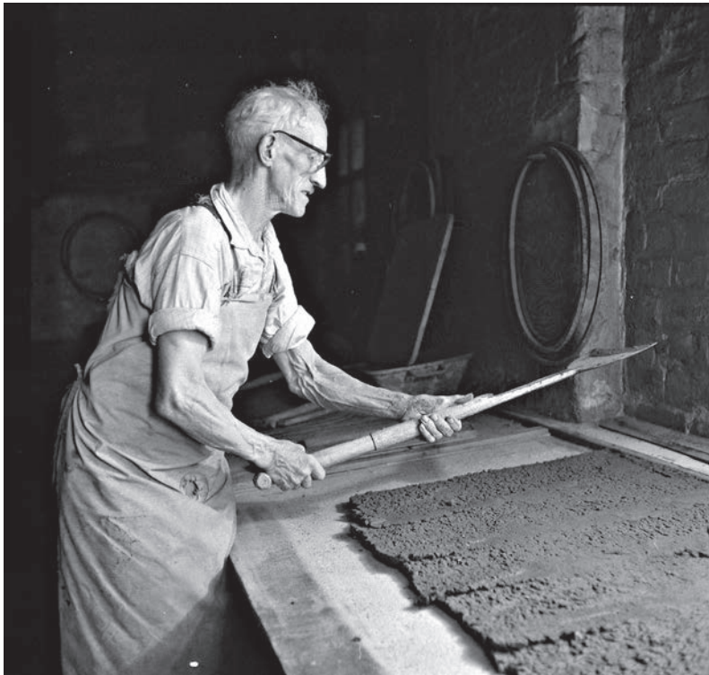
Plate 5.2. Mr. Fred Boulton using the 'grafter' to flatten down individual strips of side-marl into the frame. It would then be beaten using the mau'. Photographed at the Burgess and Leigh Factory, Middleport 1964. (Photo by and reproduced courtesy of Mr. Donald Morris).
