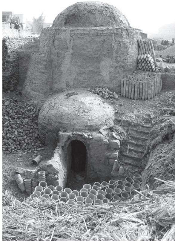
Plate 4.5. A pottery kiln at Fustat, Cairo. The lower of the two domed structures is covering the pit in which both firing and cleaning out take place, the uppermost is the tower structure into which the stacked vessels are placed for firing (see Plate 4.6). Photographed in 1998 at the workshop of Ahmed Abu Hassan. (Photo: P.T. Nicholson, courtesy of Ahmed Abu Hassan).
