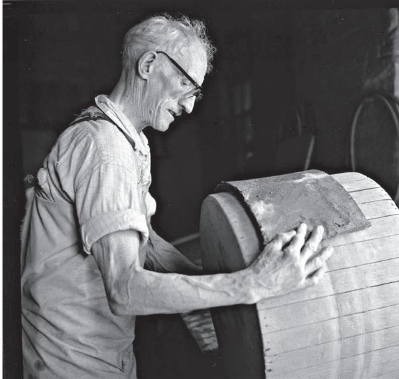
Plate 5.5. Mr. Fred Boulton rolling a strip of side-marl onto a wooden drum. Photographed at the Burgess and Leigh Factory, Middleport 1964. (Photo by and reproduced courtesy of Mr. Donald Morris).
