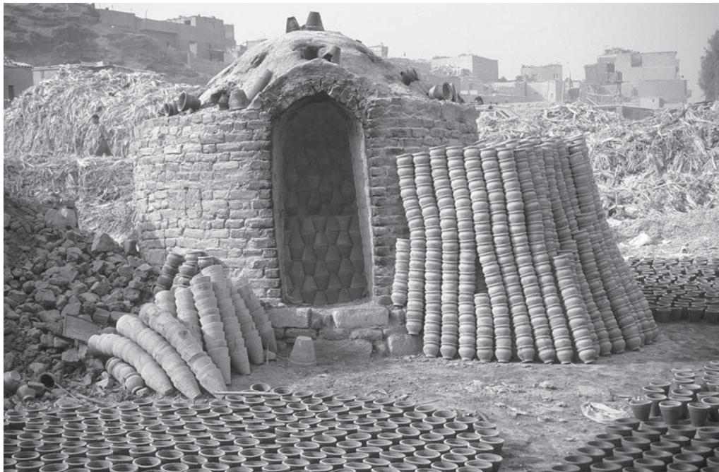
Plate 4.6. A pottery kiln at Fustat, Cairo (the same one as in Plate 4.5) showing the domed tower structure into which the pots are placed for firing, via the entrance door. No saggars are used in this industry. Photographed in 1998 at the workshop of Ahmed Abu Hassan. (Photo: P.T. Nicholson, courtesy of Ahmed Abu Hassan).
