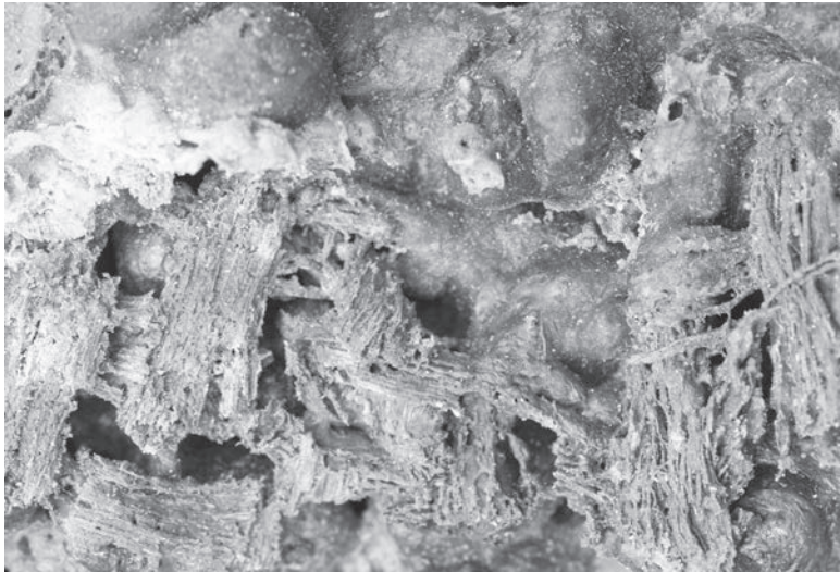
Plate 4.9. (A) Slag (V-22) preserving the impression of woven matting. (B) Detail of the weave. (Photo: P.T. Nicholson).
