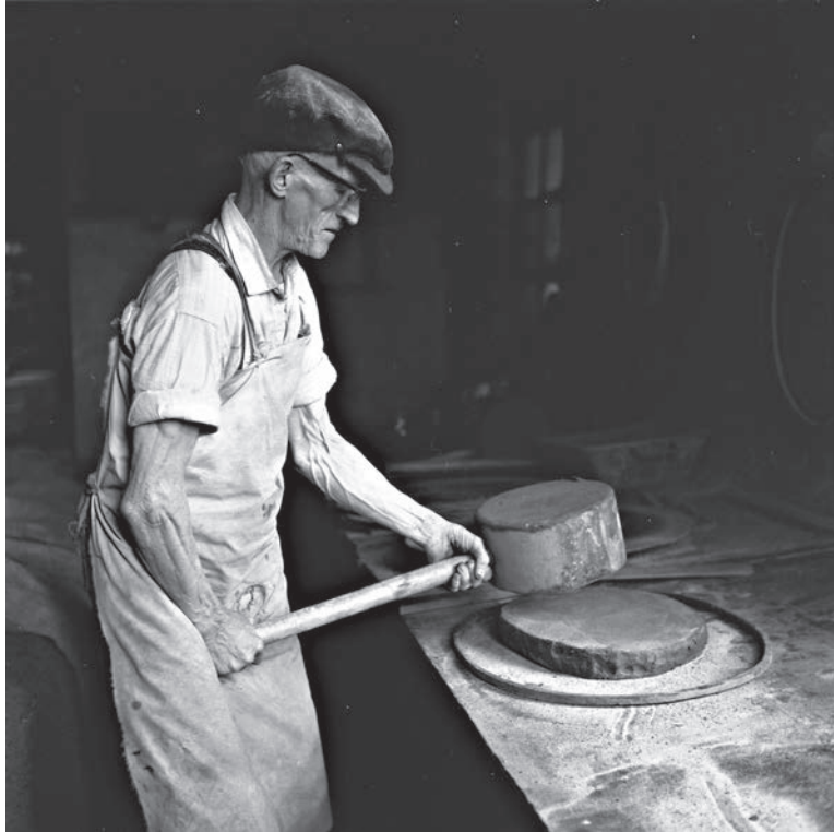
Plate 5.3. Mr. Fred Boulton using the wooden mau' to flatten bottom-marl into a circular metal frame used for making the saggar base. The mau' is also used to flatten side-marl. Photographed at the Burgess and Leigh Factory, Middleport 1964. (Photo by and reproduced courtesy of Mr. Donald Morris).
