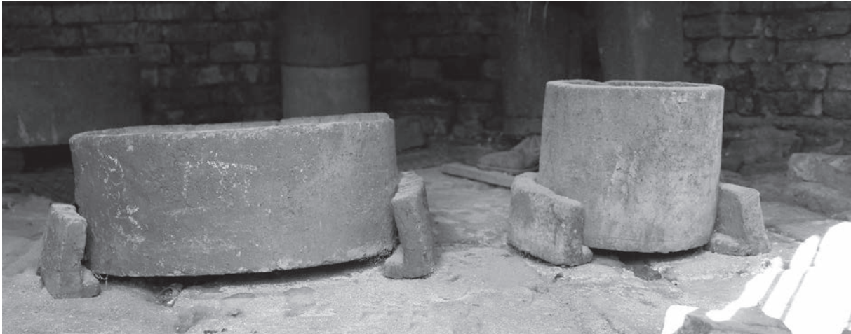
Plate 5.13. Saggars at Nantgarw Pottery, South Wales, resting on L-shaped supports to allow hot air to circulate beneath them. (Photo: P.T. Nicholson. Reproduced Courtesy of the Nantgarw Museum).
