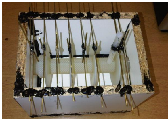
Figure 6-9. Moulding box with the SLA model in position for the manufacturing of silicone rubber moulds.
