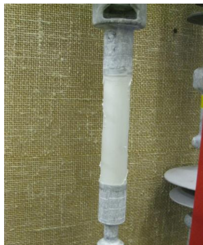
Figure 3-13. Cylindrical silicone rubber prototype with no sheds.
