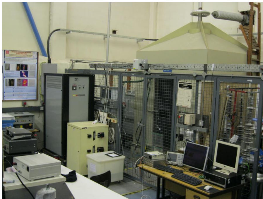
Figure 3-1. Cardiff University high voltage laboratory fog chamber.
