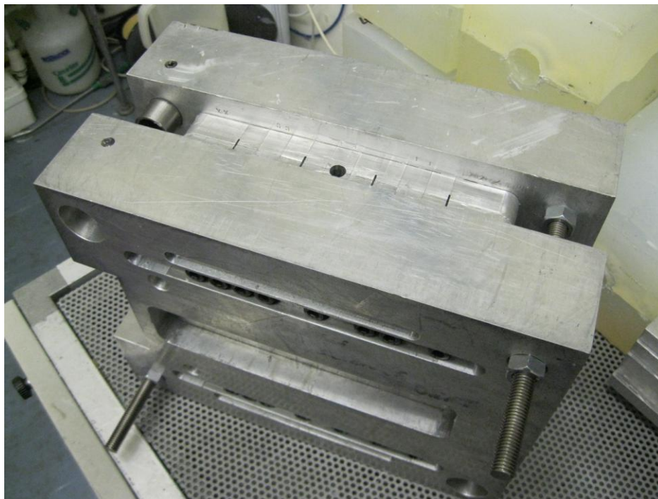
Figure A-2. The mould ready for casting.
