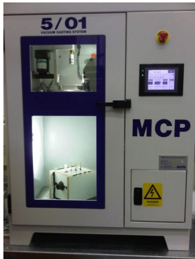
Figure 6-10. Secondary degassing in the vacuum casting machine (left). A mould for cylindrical samples during secondary degassing in vacuum, showing the trapped air escaping the silicone rubber (right).
