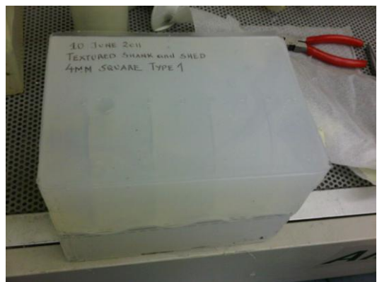
Figure 6-12. Clearing the ventilation and injection channels (left) and a completed silicone mould (right).
