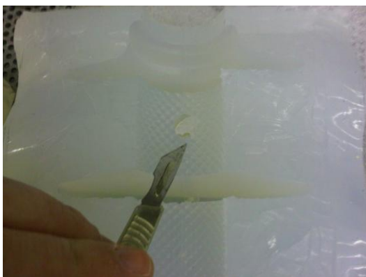
Figure 6-12. Clearing the ventilation and injection channels (left) and a completed silicone mould (right).
