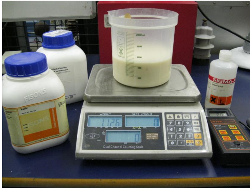
Figure 3-11. Kaolin and sodium chloride suspension with Triton X-100 wetting agent.
