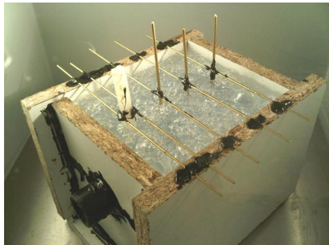
Figure 6-10. Secondary degassing in the vacuum casting machine (left). A mould for cylindrical samples during secondary degassing in vacuum, showing the trapped air escaping the silicone rubber (right).
