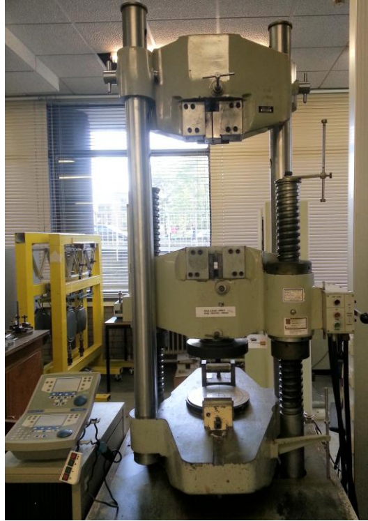
Fig 8.1 Tensile tester used to evaluate Young`s modulus of the CGO and HiB steel.
