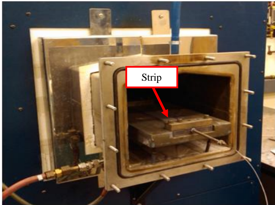
Fig 9.2 Stressing rig placed inside a retort furnace.
