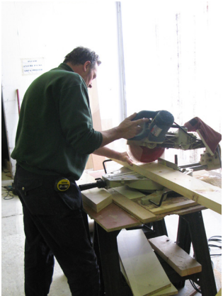
a) 150x50mm Sitka Spruce is planed on all four sides and trimmed to length and angle using a mitre saw.
