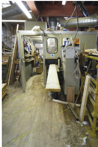
b) Plane and mould web timber to give a section of 150 x 40mm with tapered tongues to each long edge.
