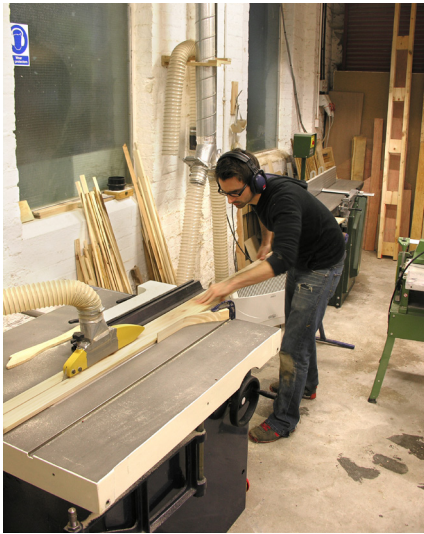
b) Timber section is ripped at 55mm and received by a roller stand on exit. The timber spring ensures that the timber is pressed firmly against the guard throughout its length with the operator inserting the timber and receiving the timber at the other end. The 55mm timber section is stacked ready for trimming to length.
