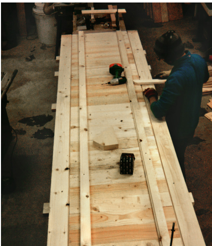
g) With open panel removed, the jig is employed to manufacture additional sheathing boards. Spruce half lap boards are set out in jig and longitudinal rails are located and clamped in place.
