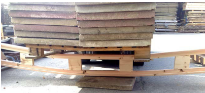
Figure 6.46: Test 3 performed at Kenton Jones Joinery. Source : Burroughs, Ladder Beam Testing Summary (Cardiff: Burroughs, 2009), pp. 7-8.
