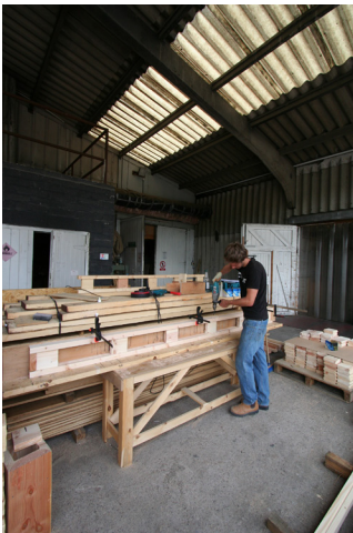
f) Slot the prepared top flange onto the tongues of the web timbers and clamp upper flange to back board
