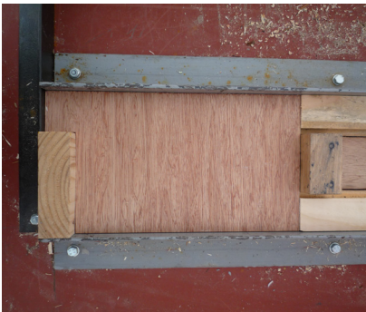
Figure 9.77: A solid timber plate is inserted into the jig to set out the geometry of a notched ladder beam formed with; a) an extended top boom and inset end web. b) a notched plywood end section reinforcing an extended top boom.
