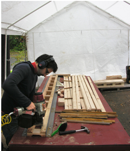
f) Starting at the open end nail through boom timbers at a slight angle into steel table to crimp nails. Pneumatic nail gun is held with a relaxed arm and nails fired to the drawing pattern as shown in dwg...
