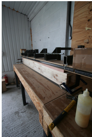
i) Once cured remove from press, remove excess glue and trim box section to length.
