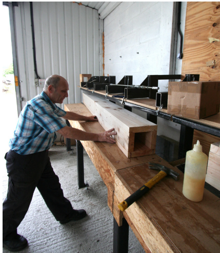
g) The upper flange is located onto the tongues of the web timber and the assembled box pushed into the press, against rear uprights.
