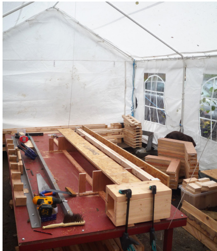
a) A jig is prepared using plywood fins and a box section. A ladder beam, prepared with joist hangers, is dropped into the plywood fin and pushed under the box section stop.
