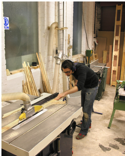
d) The second pass removes the excess of the half lap profile ensuring both sections are 55mm wide with a tolerance of \pm 1\text{mm} .
