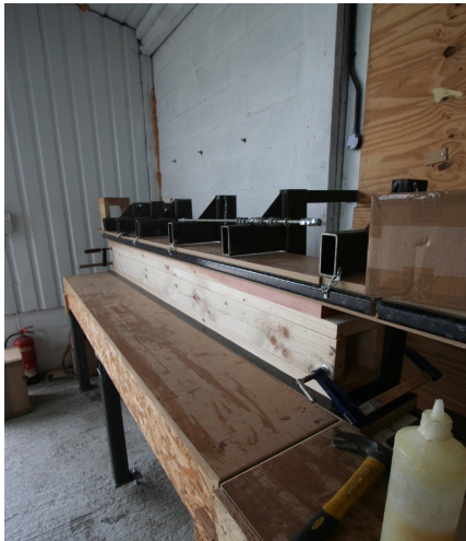
i) Once cured remove from press, remove excess glue and trim box section to length.
