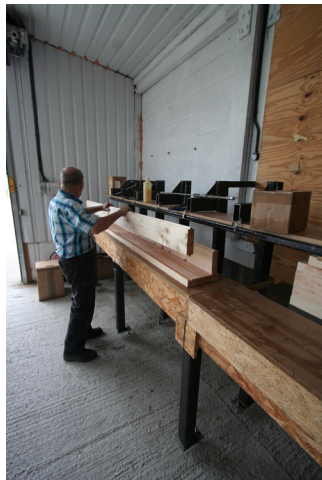
e) Web timbers are dropped into the profiled grooves.
