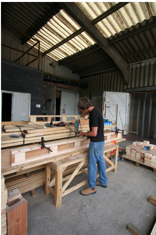
g) Pilot drill and drive 2 screws through top flange into each web timber at marked locations
