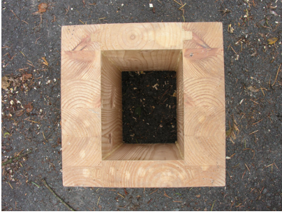
Figure 6.36: 6 50x35mm sections are laminated along the face with 125x35mm profiled web timbers
