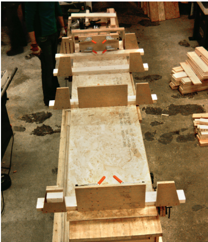
a) The jig is set up on the standard workshop benches comprising four plywood fins, notched to receive and restrain ladder beams.
