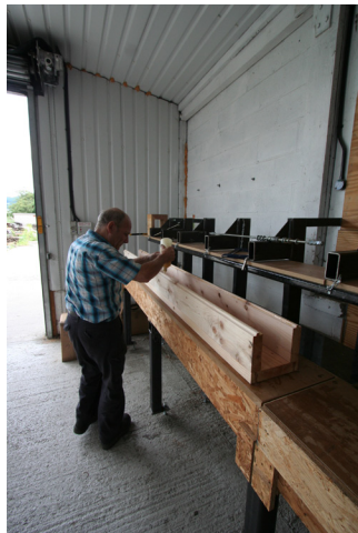
f) The tongue and groove profile holds the assembled box stable and square during assembly. Adhesive is then applied to the upper edge.
