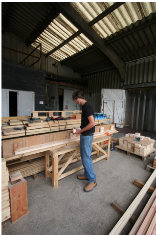
e) Slot web timbers into groove of the bottom flange at marked locations
