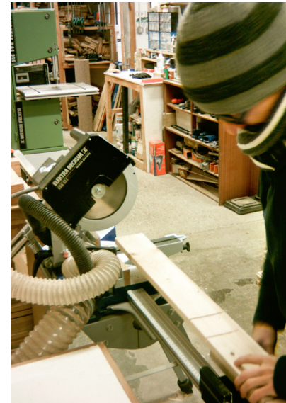
Figure 9.76: Cutting boom timber to length using a mitre saw. A timber measuring stick with end stop is used as a length gauge.
