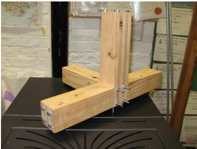
Figure 9.39: Bolted timber multi direction connector proto-typed at half scale
