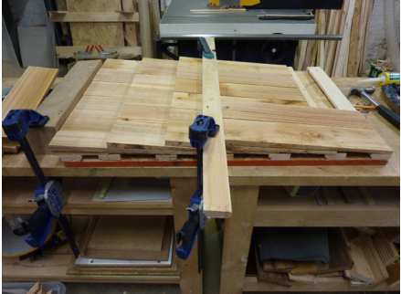
b) A timber batten is employed to maintain a straight edge to the exposed end of the shingle.
