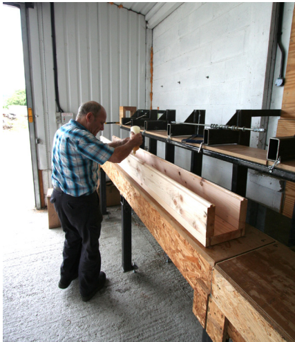
f) The tongue and groove profile holds the assembled box stable and square during assembly. Adhesive is then applied to the upper edge.
