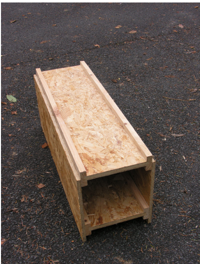
Figure 6.51: Preliminary trials with spruce based box panels using solid web joists with t+g internal and external linings. Figure 6.52: Proposed geometry has male and female junctions to form a simple stacking junction. Figure 6.53: OSB based alternative box panel.
