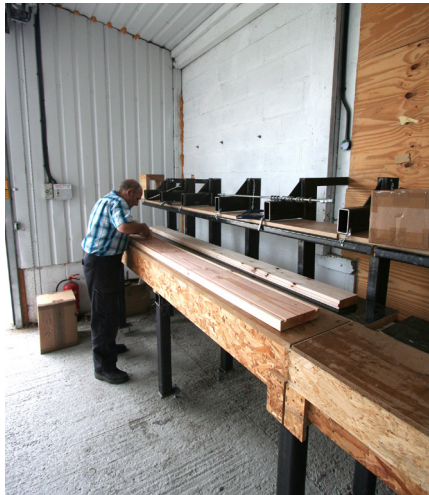
d) Working immediately adjacent to the press on an extended table, polyurethane glue is applied to the prepared grooves in the bottom flange.
