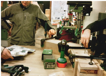
f) Whilst clamped pilot holes are drilled and 4 no 80mm screws driven through the laminations. Once cured, the clamps are removed and a further 3 screws driven in from the opposite face.
