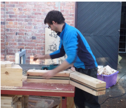
Figure 9.74: Sliding connector into box section hollow.
