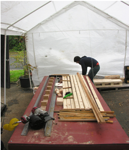
a) The jig is prepared with oak separator blocks in place and cut timbers placed around the table. Table must be clear of timber chippings and dead knots.
