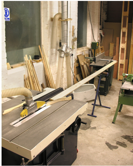
a) The table guard is set to 55mm and a timber spring is clamped to the table base to exert pressure on the timber section. A roller stand supports the timber section.
