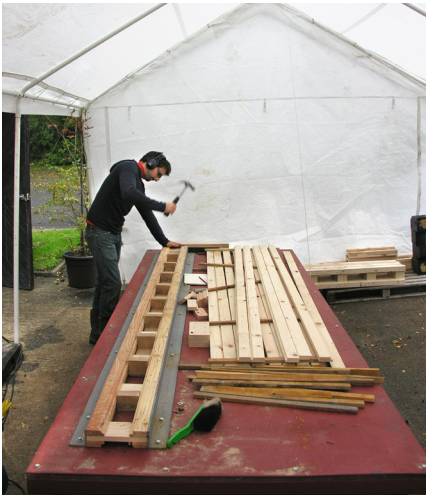
g) Ladders are then tidied up manually to ensure that nail heads and crimped ends are suitably bedded into timber, particularly where nails have 'bounced back' off table.
