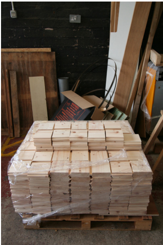
a) Web timbers are profiled as full length timbers, typically taken from rejected box section material, and cut to length.
