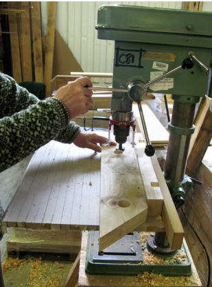
b) Timber 'cheek's are predrilled, first with a 16mm drill, then a 30mm augur to accommodate the nut and bolt head within the timber section.
