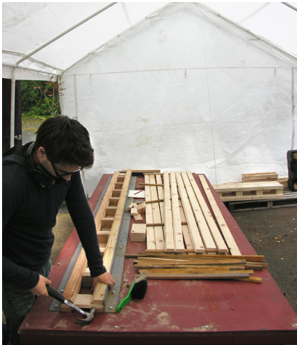
e) Place boom timbers into jig, half lap edges face into the centre of the ladder. Tap against table and end stop to ensure tight fit, cut booms act as a length gauge for accuracy.
