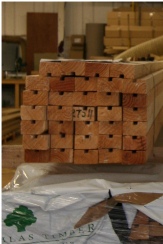
b) Flange timbers with profiled groove to receive web timbers, cut to length and visually assessed for distortion and quantity and size of knots.
