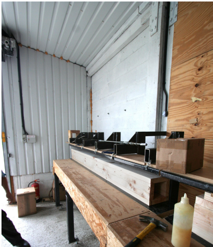
h) Filling the hose line with air using a small industrial compressor lifts the table bed and compresses the box against the top restraints of the presses. Clamps to the rear uprights ensure the section is square.
