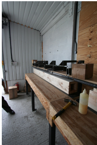
h) A compressor fills a doubled line of fire hose to lift the table bed and compress the box against the top restraints of the presses. Clamps to the rear uprights ensure section is square.
