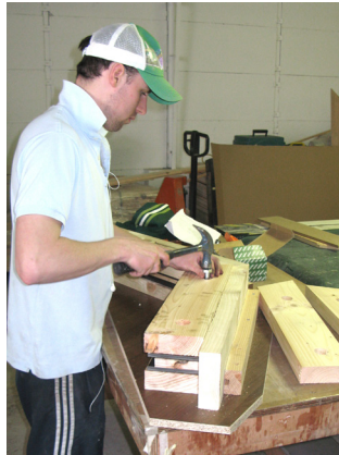
d) Once located tap through 4 no M16 bolts and washers, turn over and apply washers and nuts.
