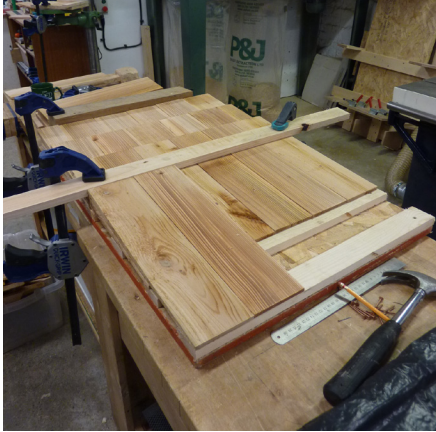
c) Shingles are cut to length and predrilled to receive non corrosive fingers.
