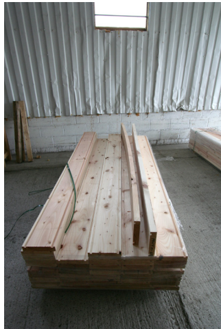
c) Plane and mould the flange timber to give 2 sections of 210 x 40mm with 2 longitudinal grooves.
