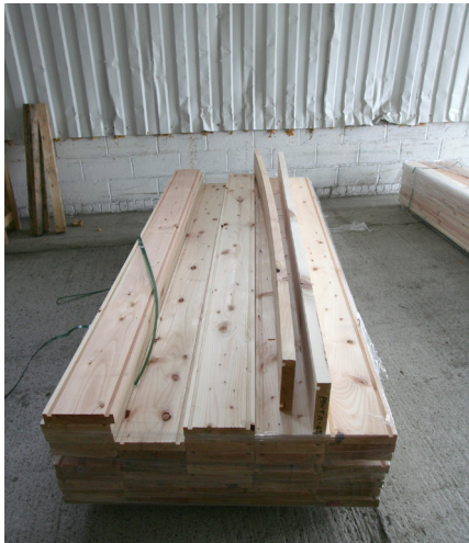
c) Plane and mould the flange timber to give 2 sections of 210 x 40mm with 2 longitudinal grooves.
