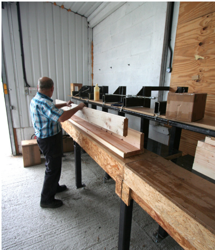
e) Web timbers are dropped into the profiled grooves.
