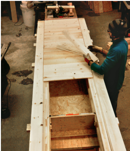
e) Cut to width and thickness, half lap spruce boards are slotted laterally into the jig, sitting on the top flange of the ladder beam.
