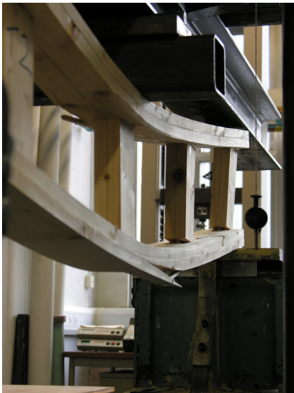
Figure 6.44: Closeup of failure of simulated OSB flange and significant rotation of struts under loading.
