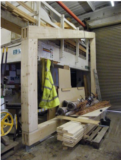
Figure 6.23: Portal frame arrangement employed by Cowley Timberwork to test deflection under horizontal loading, ie wind loads.
