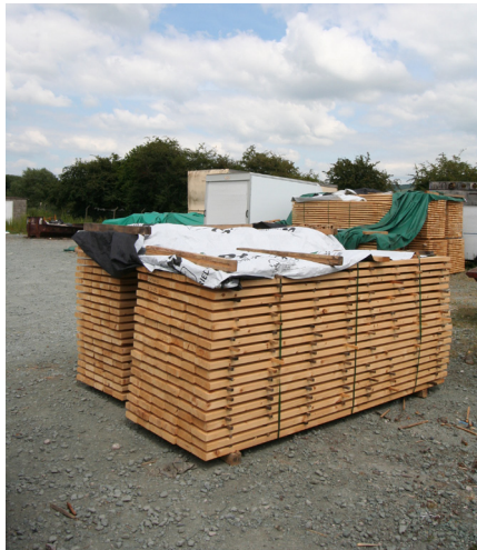
a) Select 2 lengths of standard C16 Sitka Spruce 225 x 47mm for flange timbers and 2 lengths of 150 x 47mm for web timbers.
