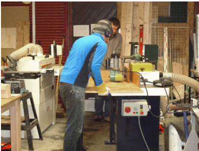
Figure 9.85: 18mm OSB sheathing boards are passed through a spindle moulder to route a 9mm groove to each long edge.
