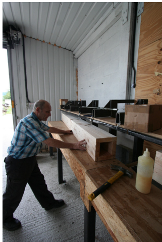
g) The upper flange is located onto the tongues of the web timber and the assembled box pushed into the press, against rear uprights.
