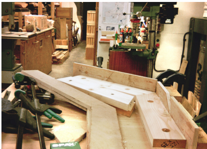
b) The first layer of plywood is used as a template to set out the jig. A layer of Polyurethane glue is applied to the plywood and the mitred timber laminates are pressed firmly into place
