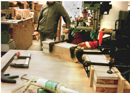
e) Clamps are applied to press laminations during curing and ensure no slippage occurs.
