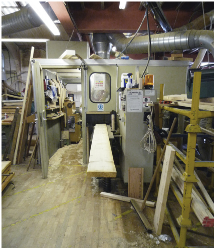
b) Plane and mould web timber to give a section of 150 x 40mm with tapered tongues to each long edge.
