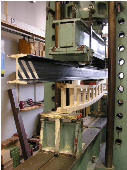
Figure 6.45: Failure of glued connection caused by significant rotation of struts.
