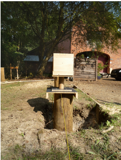
Figure 9.30: Prototype of foundation connector fabricated out of softwood and OSB to trial the geometry of fixings.
