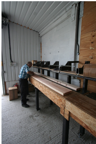
d) Working immediately adjacent to the pneumatic press on an extended table, polyurethane glue is applied to the prepared grooves in the bottom flange.
