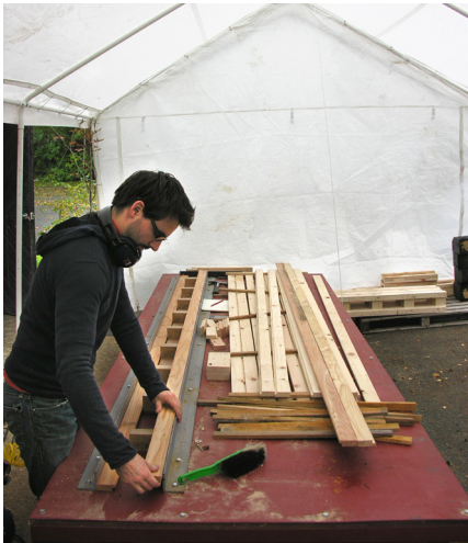
b) Place boom timbers into the jig and tap down flat against steel table and against end stop, oak spacers ensure booms are tight against steel rails.
