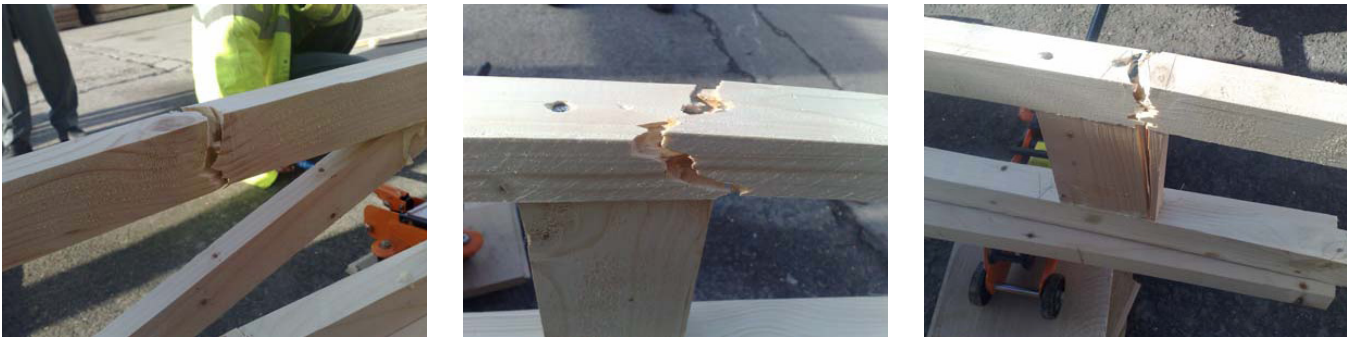
Figure 6.42: Selection of photographs of preliminary testing on ladder beams as Kenton Jones Joinery.
