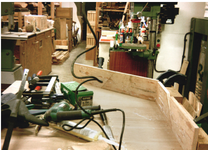
a) Blocks and plywood pieces are clamped to a sheet of plywood to create an assembly jig
