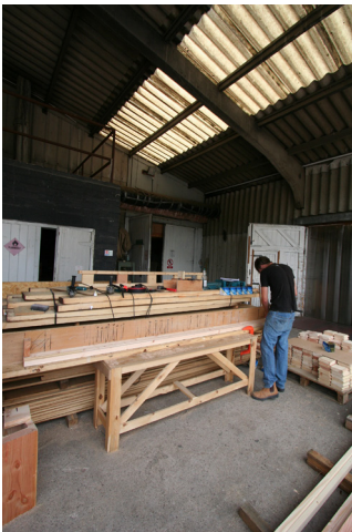
d) Place bottom and top flanges on bed of the assembly table and apply polyurethane glue to the grooves at locations set out on assembly table
