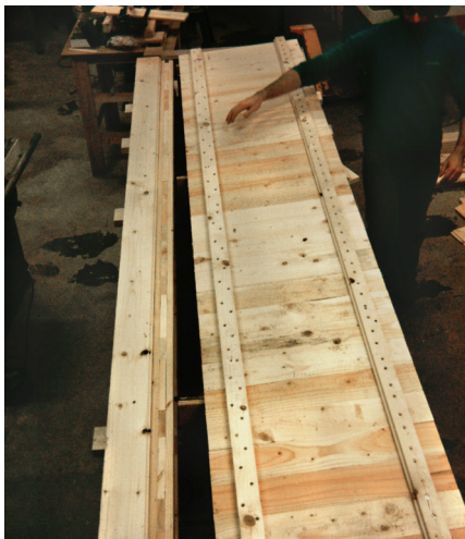
i) Panel is removed from jig and located against ladders of the open panel using the longitudinal rails. Boards are subsequently screwed into the top flange of the ladder beam.
