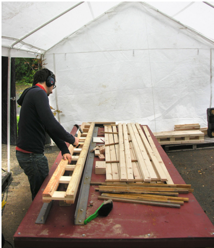
h) Remove ladder from jig using a claw hammer and remove oak spacers from between the webs. Store flat in a dry place.
