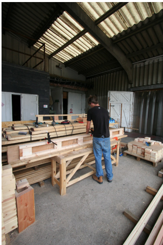
h) Remove clamps and turn ladder over. Reclamp, pilot drill and drive 2 screws into each web timber.
