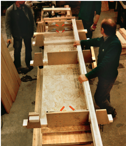
b) Ladders are installed into the notched fins and pushed up against an end stop, to the far end of the photo. Fins are spaced to receive alternative ladder lengths.
