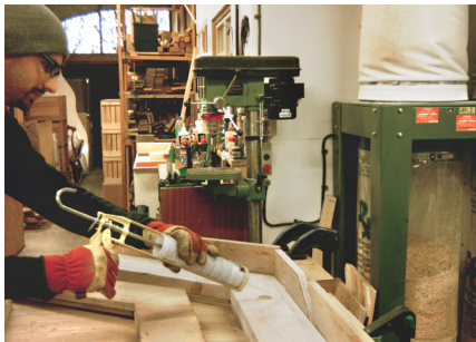
c) Glue is spread across the timber layer and a further lamination of plywood pressed in place.
