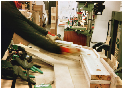
d) A second lamination of mitred timber and plywood are glued in place to complete the connector.
