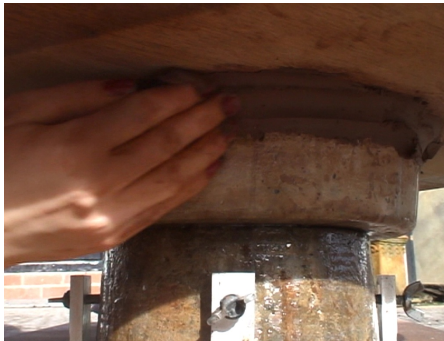
Figure 6.15: Attaching the wheelhead to the concrete wheel bearing using coils of clay. Photo: S. Doherty
