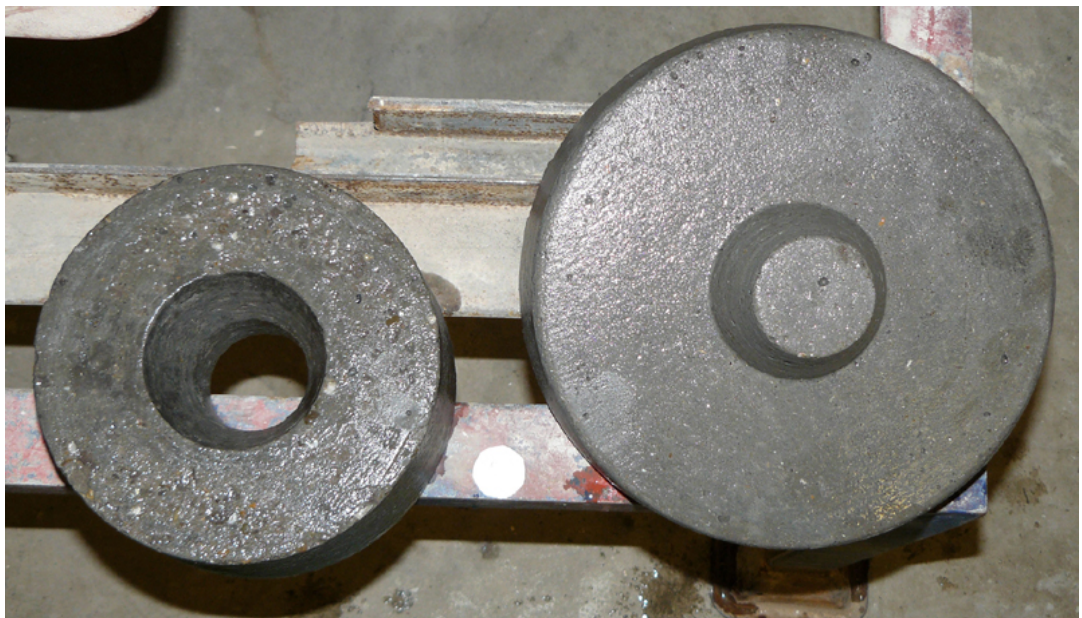
Figure 6.13: The newly cured concrete potter's wheel bearings based on the British museum example BM32622. Photo: Alan Davies
