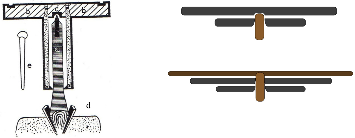
Figure 2.8: Left: Japanese potter's wheel with socketed disk (a) hardwood pivot; (b) hardwood wheel with a porcelain cup as bearing; (c) hollow cylinder extends down the pivot to provide an annual bearing at (d) which steadies the wheel; (e) stick to place into the notches in the wheelhead to spin it. Childe (1954: 195, fig 120). Right: Suggested arrangement of basalt bearings (grey), the lower example with a wheelhead (brown) attached, with a wooden pivot. Drawings: S. Doherty
