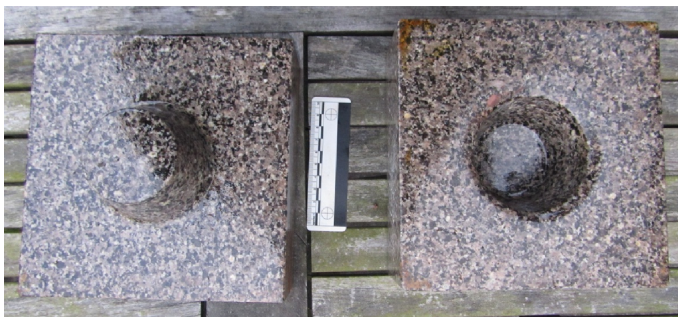
Figure 6.20: The carved and honed granite replica potter's wheel bearings. Note the lubrication discolouration already starting to form Photo: S. Doherty
