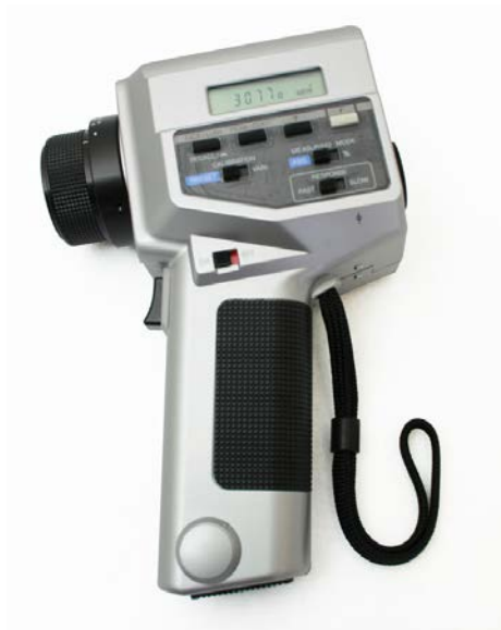
Figure 6.5 Luminance meter used for determining reflectance of surfaces
