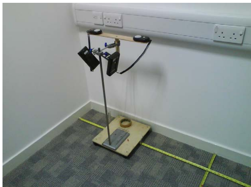
Figure 6.7 Working plane (800mm) measurement setup
