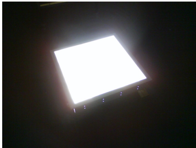
Figure 6.14 Custom LED ceiling tile type luminaire demonstrator used for measurements
