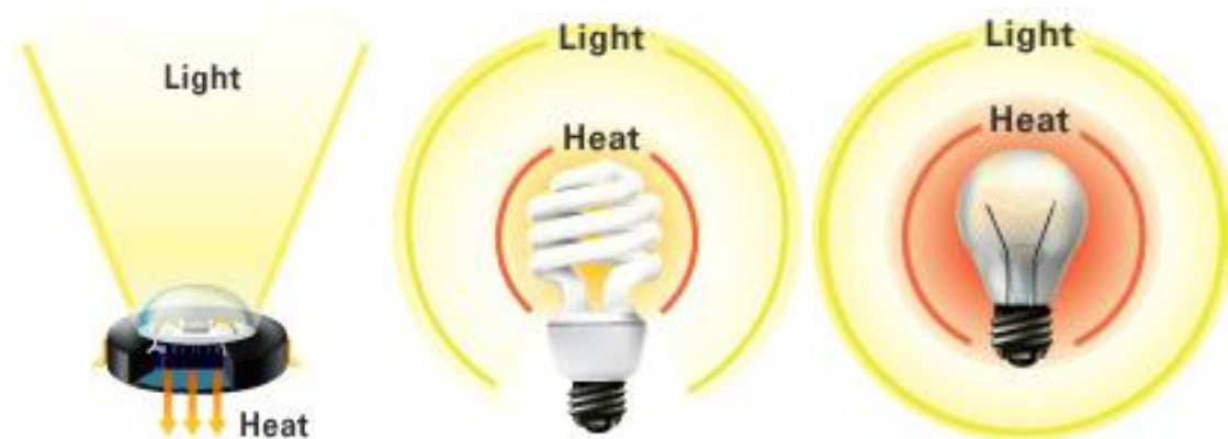
Figure 4.1 Visual comparison of light distribution between three different light sources (LED, compact fluorescent, incandescent) (source: Energy Star)
