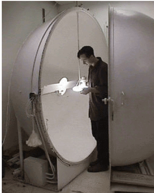
Figure 6.3 Integrating (or Ulbricht) sphere, used for measuring luminous flux of light sources (source: Lighting Research Group)
