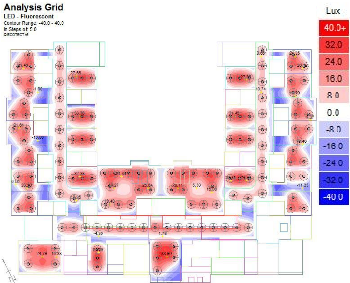
Figure 9.15 Differences in lux levels between fluorescent and LED lighting, when fluorescent lux levels are subtracted from LED lux level at each point. Blue colours indicate a deficit of lux level and red colours and surplus of lux levels compared to fluorescent. White, indicates that lux levels are exactly the same.
